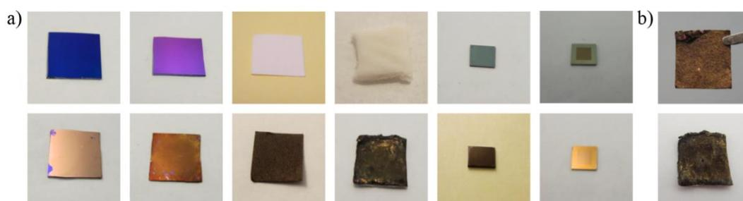
Figure 7.1: a) Representative substrates before (supports, top row) and after (bottom row) electroless gold plating. Left to right: Silicon nitride, polymer-grafted
