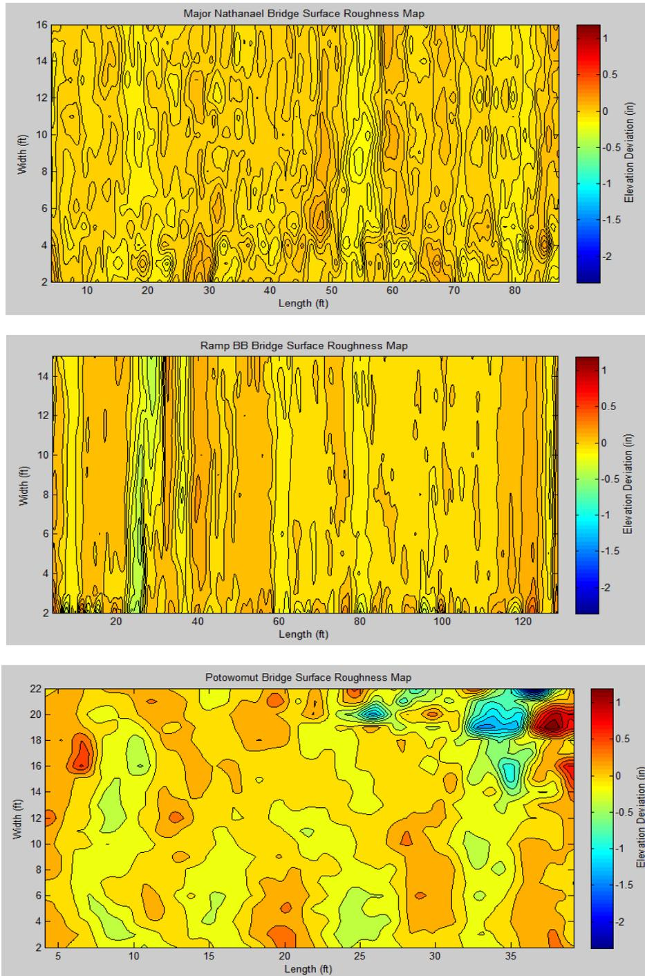
**Figure 4.1.7: Surface Roughness Mapping Comparison for Major Nathanael Greene (Top), Ramp BB (Middle), and Potowomut (Bottom)**
