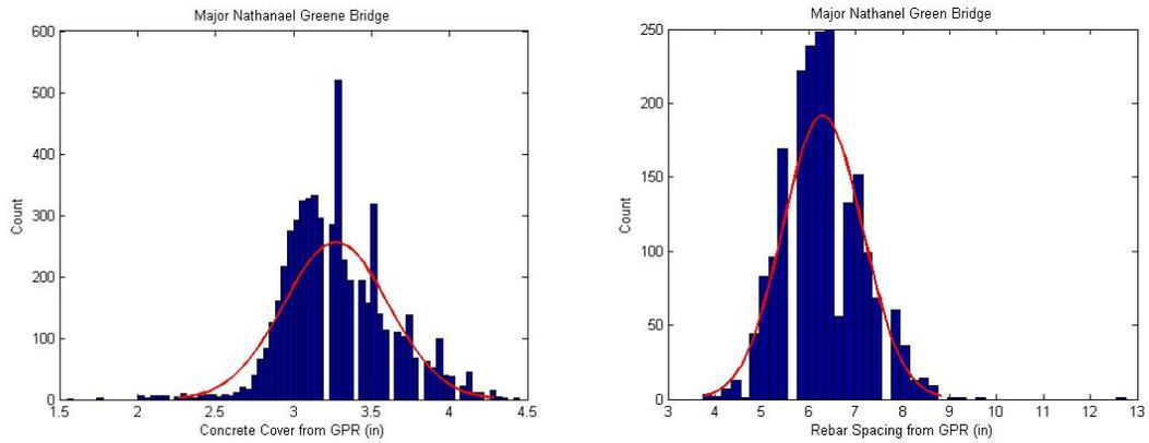
**Figure 4.2.4: Concrete Cover and Rebar Spacing Distribution for Major Nathanael Greene**
