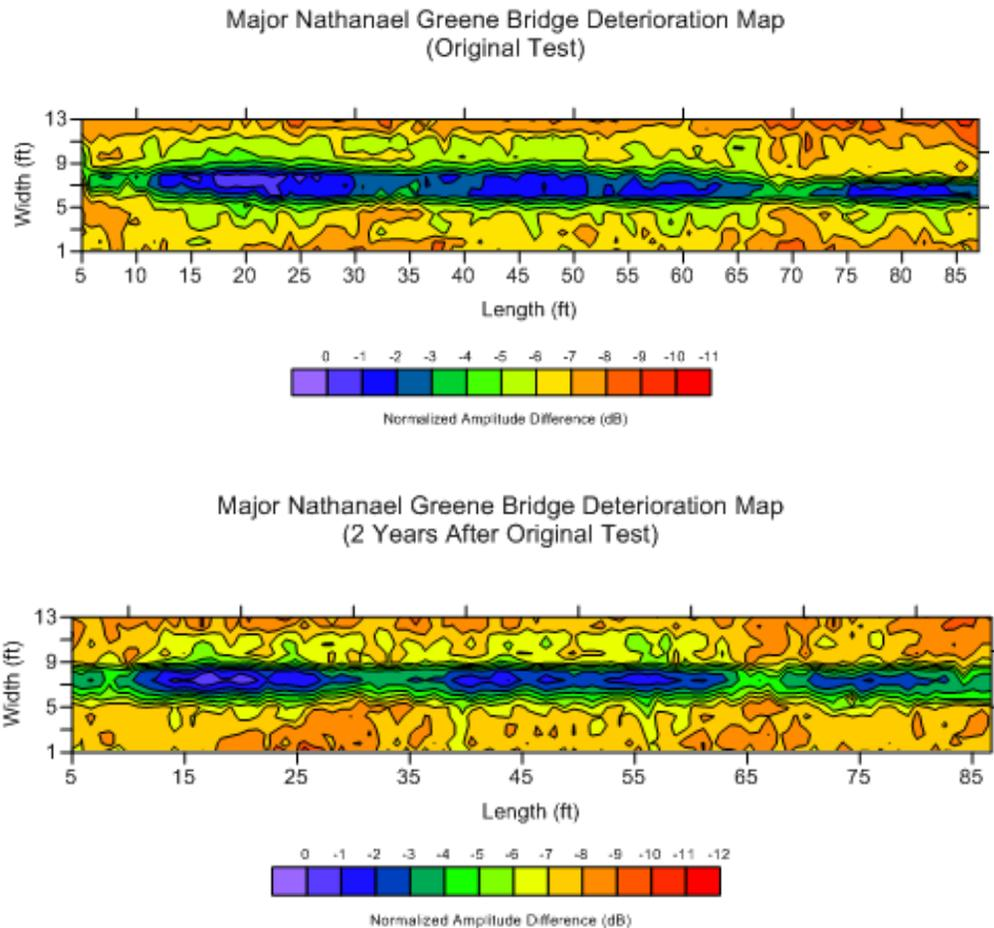
**Figure 4.4.1: Major Nathanael Greene Bridge GPR Subsurface Deterioration Map**
