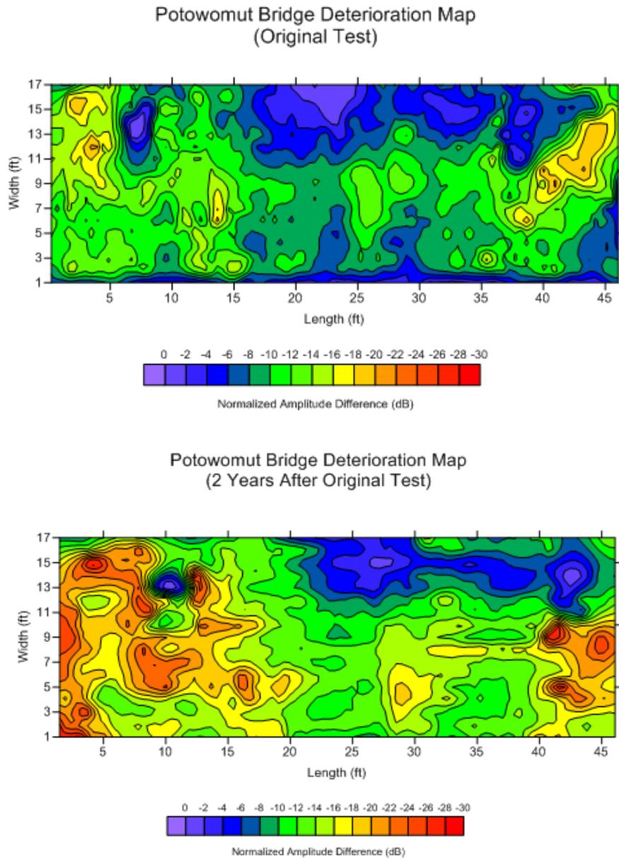
**Figure 4.4.8: Potowomut Bridge GPR Subsurface Deterioration Map Comparison**
