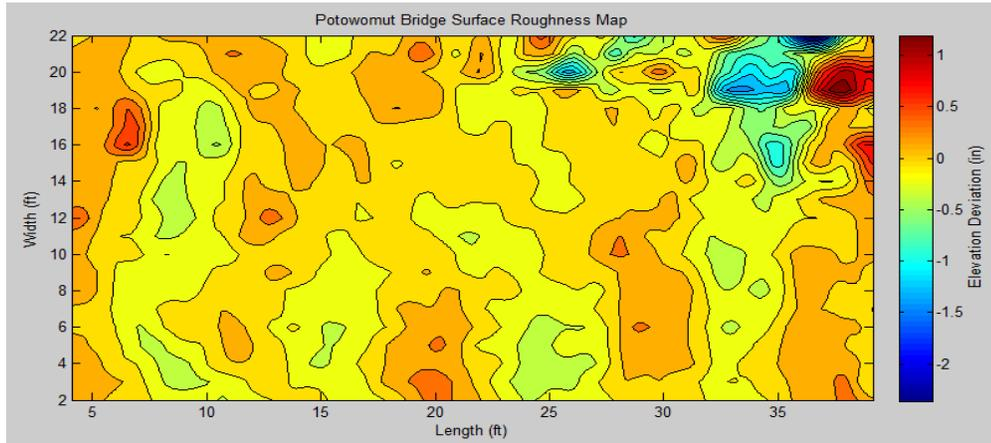
**Figure 4.1.6: Potowomut Bridge (Top) Deck Surface (Bottom) Surface Roughness Map**
