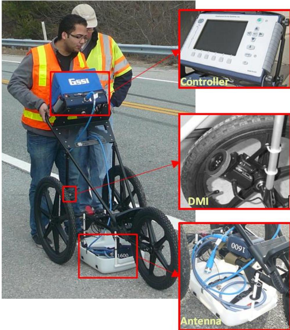
**Figure 3.4.5: Components of the GSSI GPR Equipment**
