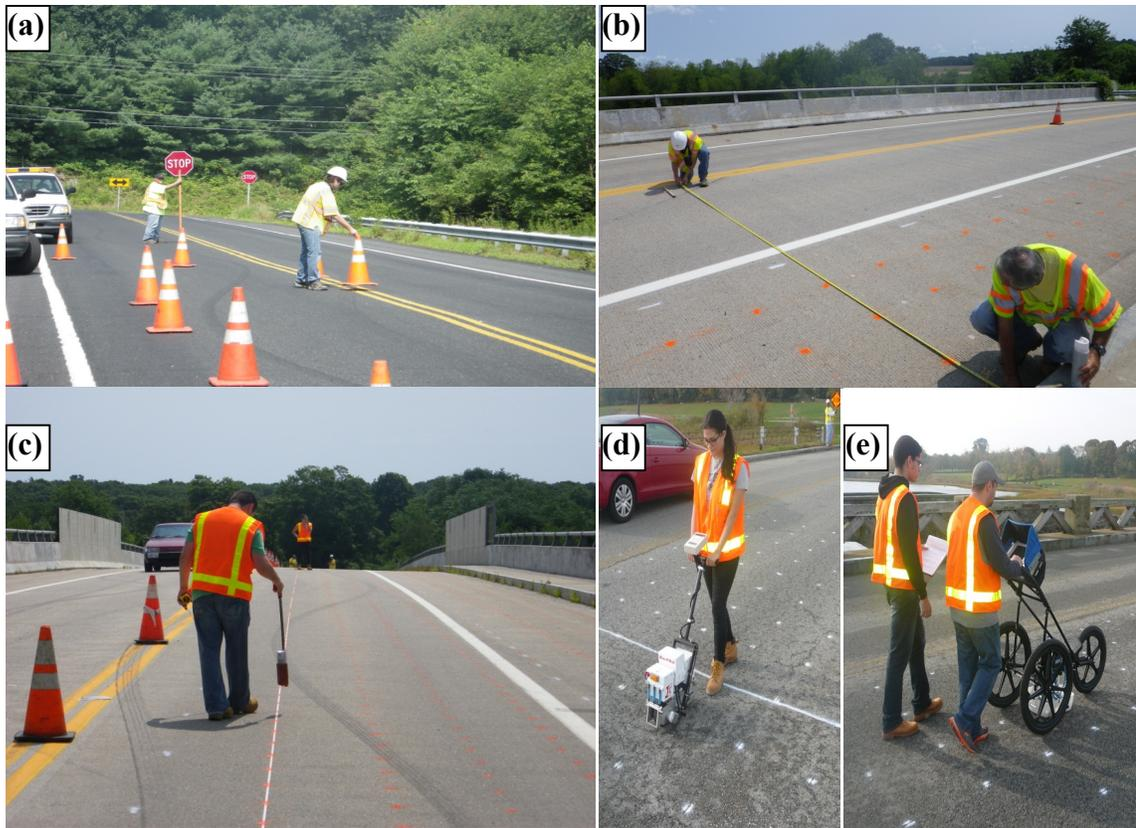
**Figure 3.4.1: Field Testing Setup (a) Lane Closure and Traffic Control (b) Transverse Grid Markings (c) Longitudinal Grid Markings (d) Data Collection with the Surface Profiler (e) Data Collection with GPR**
