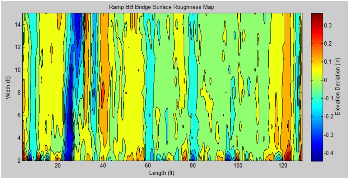
**Figure 4.1.5: Ramp BB Bridge (Top) Deck Surface (Bottom) Surface Roughness Map**
