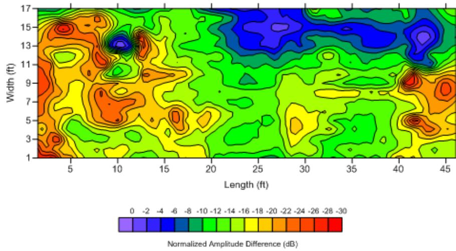
**Figure 4.4.5: Potowomut Bridge GPR Subsurface Deterioration Map**
