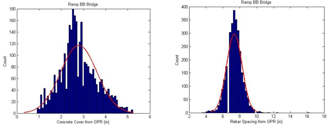
**Figure 4.2.5: Concrete Cover and Rebar Spacing Distribution for Ramp BB**
