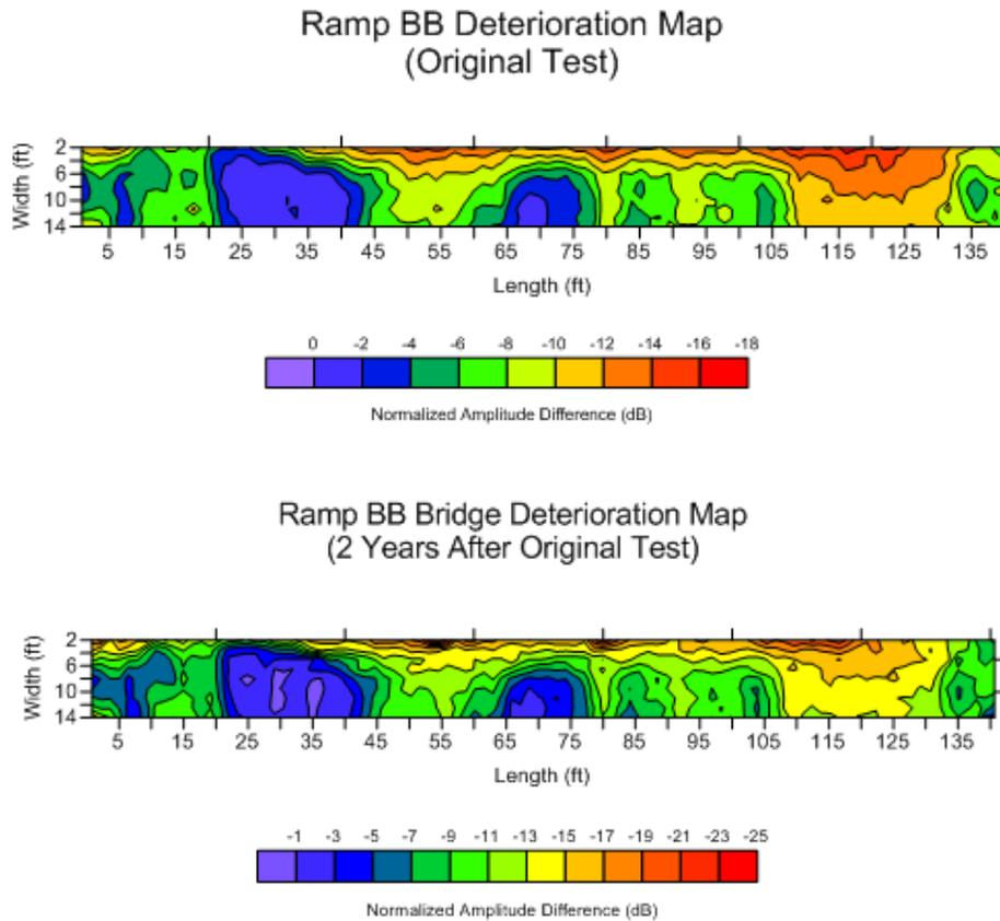
**Figure 4.4.3: Ramp BB Bridge GPR Subsurface Deterioration Map**
