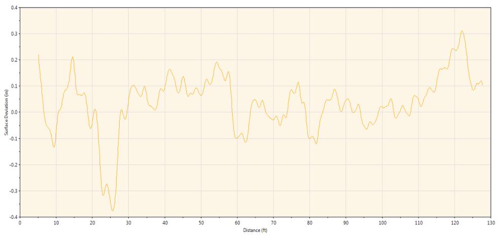
**Figure 4.1.2: Filtered Surface Profile from Ramp BB Bridge at 2 ft from Curb**
