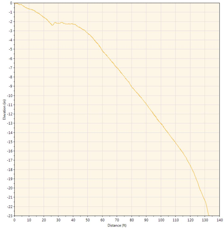
**Figure 4.1.1: Raw Surface Profile from Ramp BB Bridge at 2 ft from Curb**
