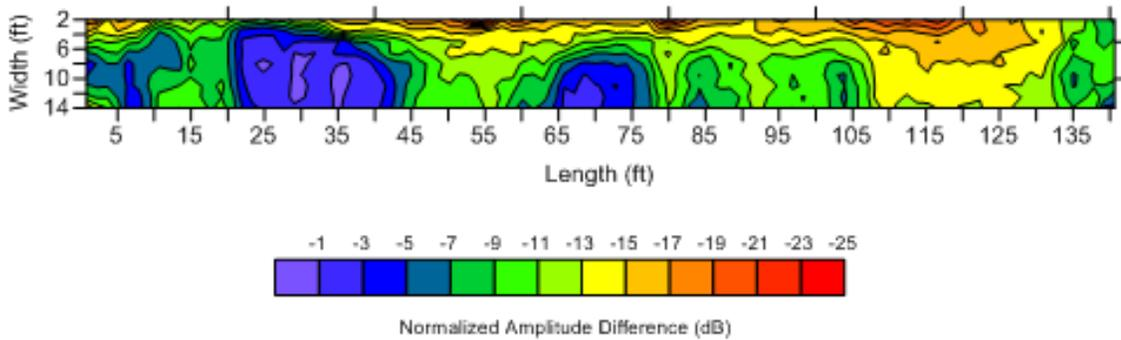
**Figure 4.4.7: Ramp BB Bridge GPR Subsurface Deterioration Map Comparison**
