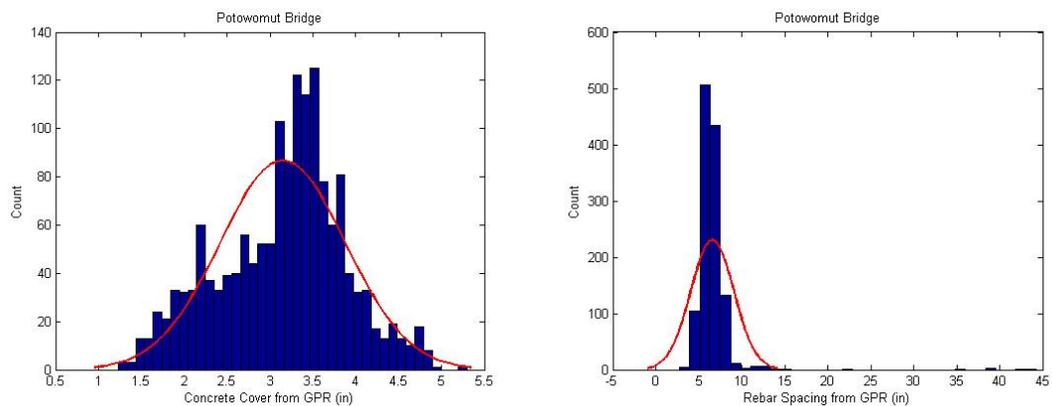
**Figure 4.2.6: Concrete Cover and Rebar Spacing Distribution for Potowomut**
