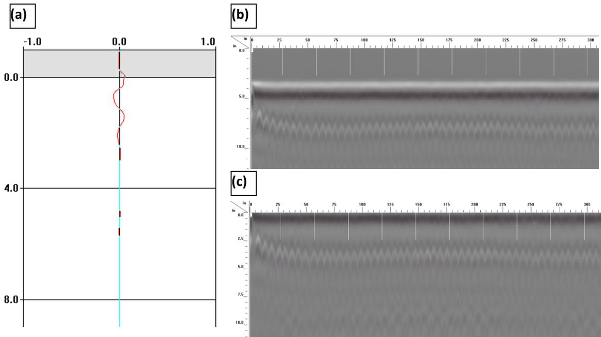
**Figure 4.2.1: Time Zero Correction (a) A-scan (b) Data Before Time Zero Correction (c) Data After Time Zero Correction for the Major Nathanael Greene Bridge**
