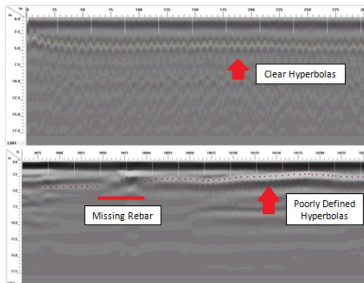
**Figure 4.3.1: Rebar Location in GPR Scans from (a) Major Nathanael Greene Bridge and (b) Potowomut Bridge**
