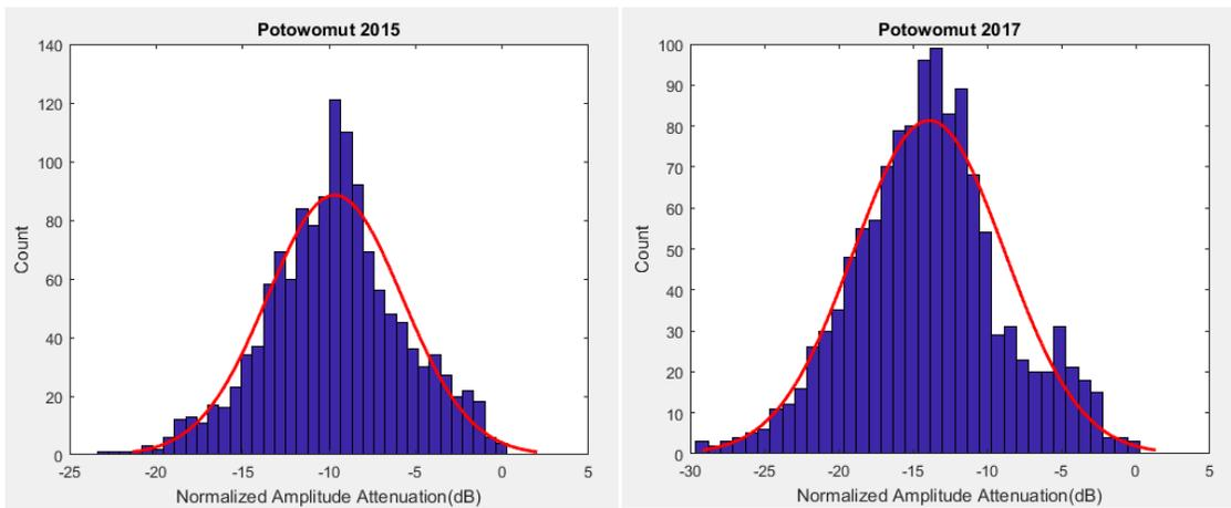
**Figure 4.4.11: Potowomut Attenuation Histograms for 2015 and 2017**
