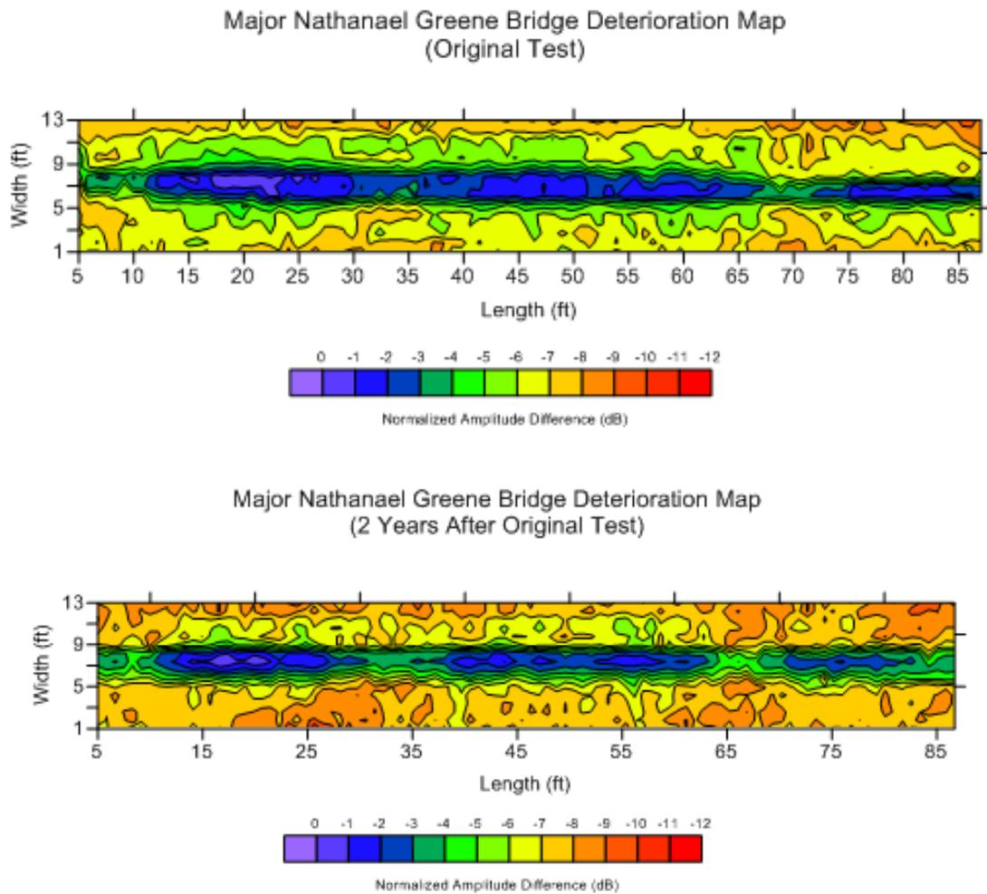
**Figure 4.4.6: Major Nathanael Greene Bridge GPR Subsurface Deterioration Map Comparison**
