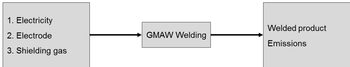
Figure 35: Input-Output diagram of GMAW Welding
