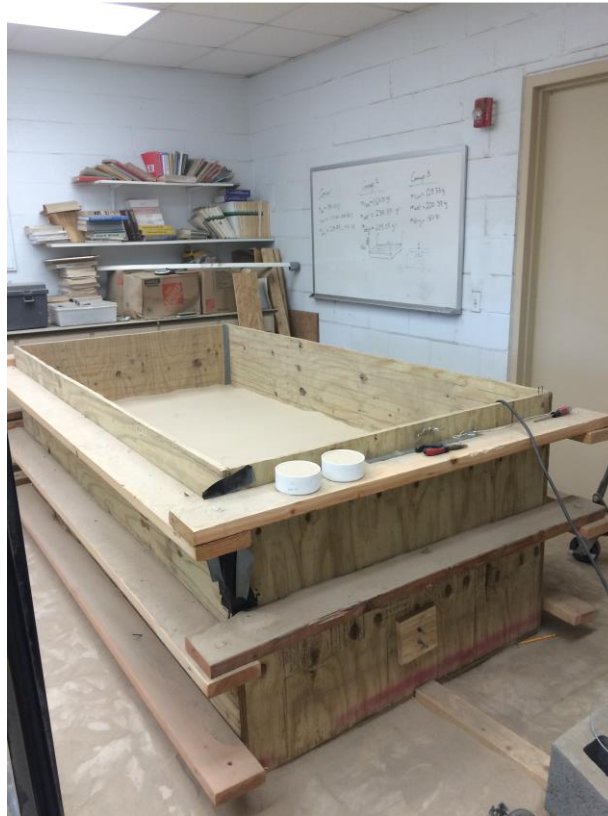
Figure 14: Test Tank for static penetration tests; note the white cups measuring in-place unit weight
