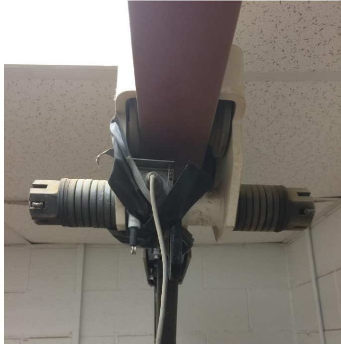
Figure 15: Celesco String Potentiometer mounted on the frame
