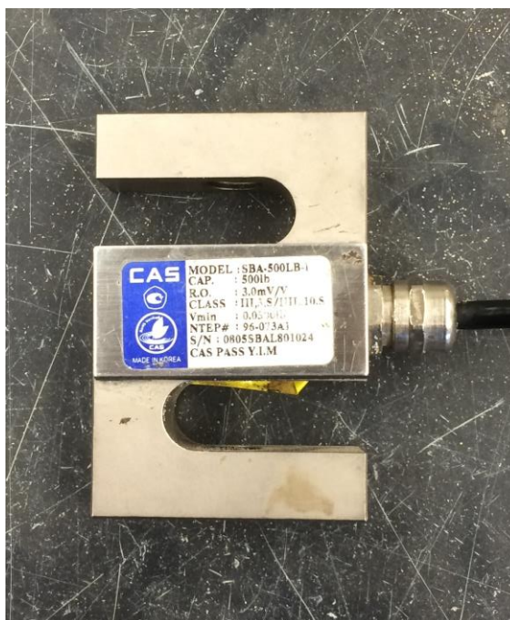
Figure 16: Load Cell Omega SBA-500LB
