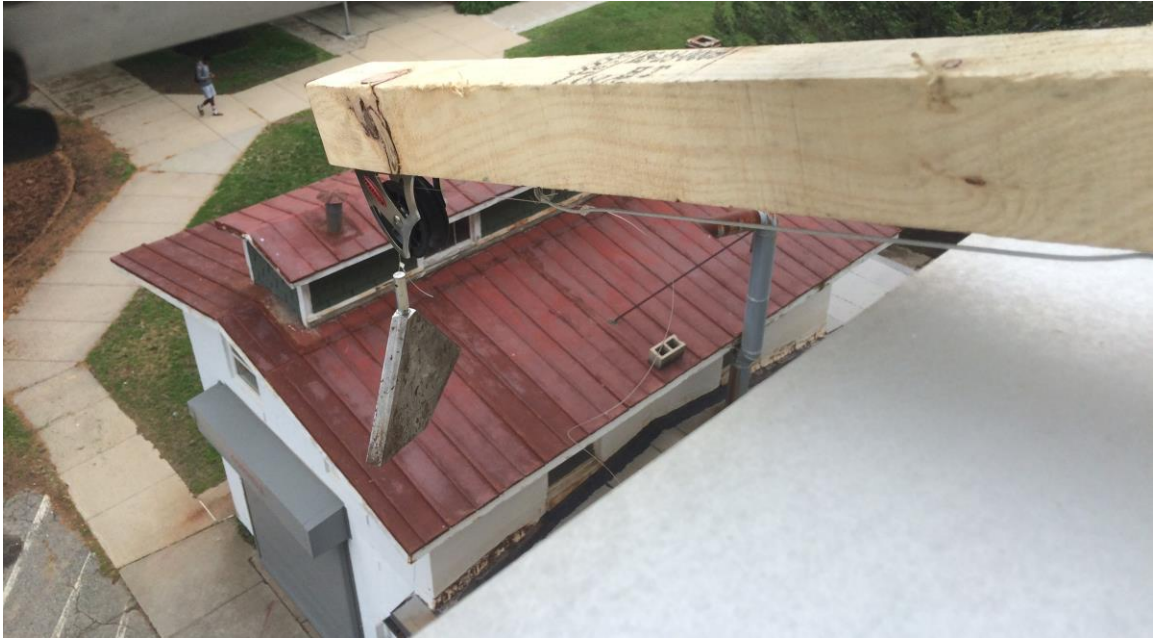
Figure 24: Test Set Up for the outside Tests. View on anchor and pulley
