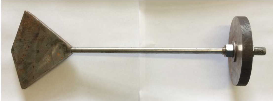
Figure 12: Anchor blunt edge with attached rod and added weight
