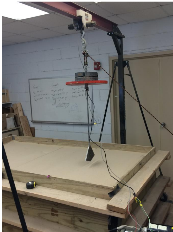
Figure 20: Picture of Test Set Up for Static Penetration Test
