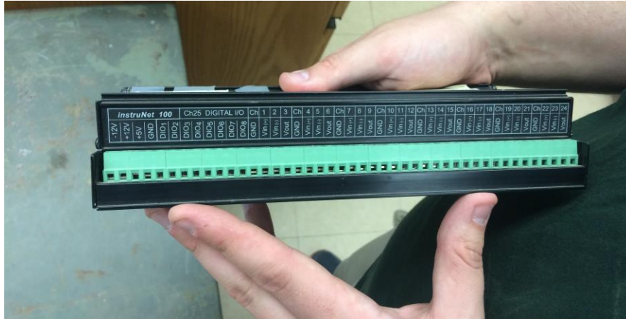
Figure 17: Data Acquisition System Omega InstruNet 100
