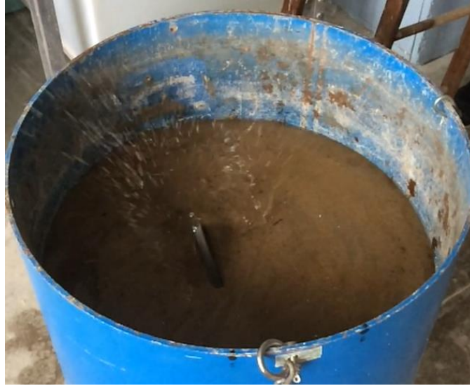
Figure 29: Penetration of the blunt edge anchor at the moment of impacting into saturated sample
