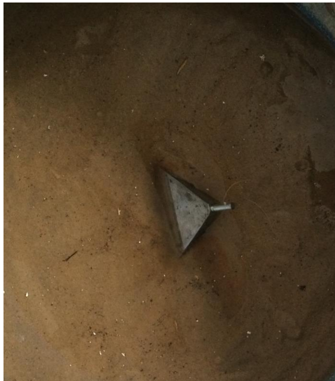
Figure 30: Final Position of the blunt edge anchor after penetrating into saturated sample
