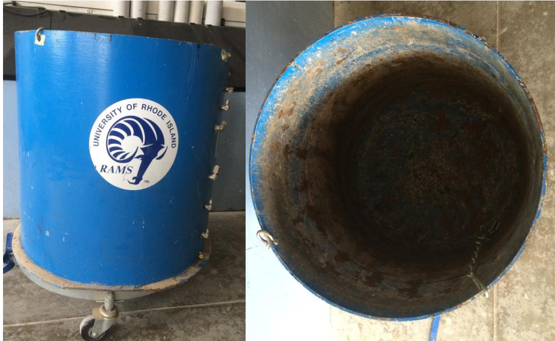
Figure 21: Test tank for dynamic penetration tests
