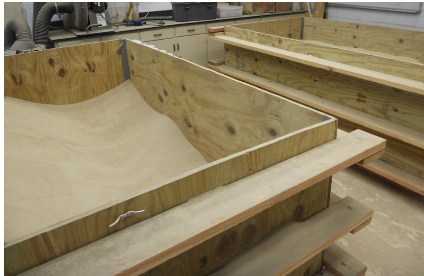
Figure 18. Photograph of the 1g-test tank (right) and the storage tank (left) at URI.
