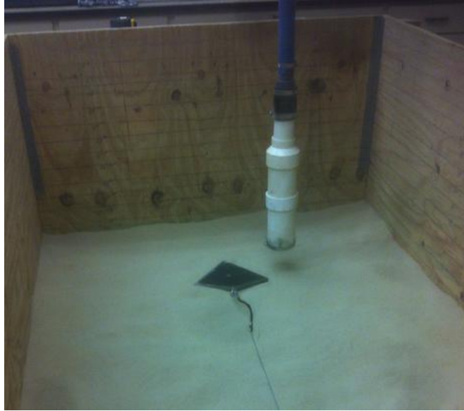
Figure 46. Photograph of the test anchor for the in-plane shear (horizontal fluke) tests.
