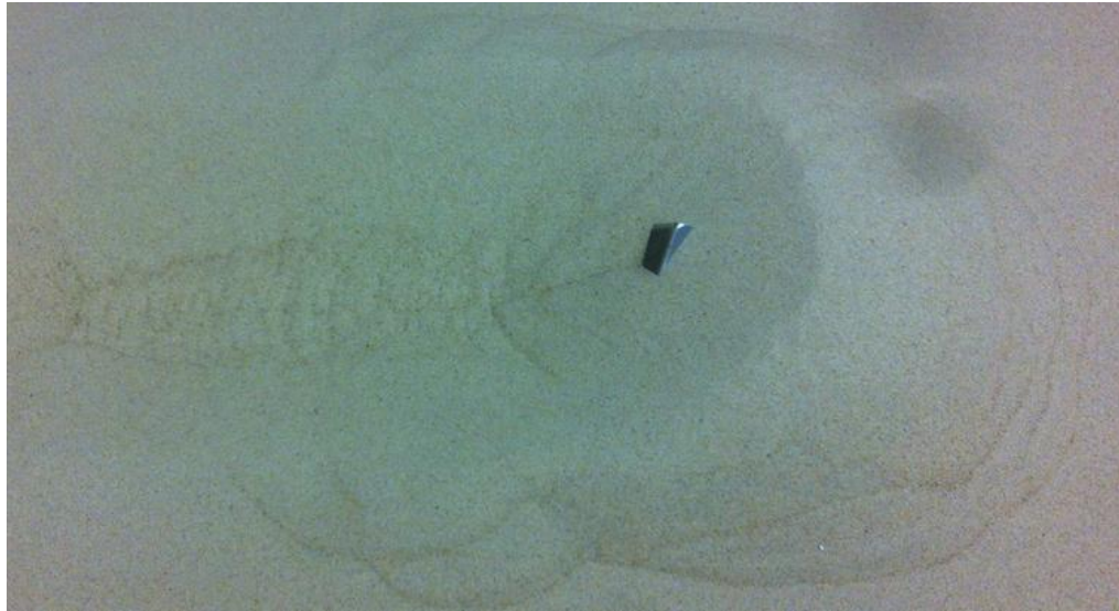
Figure 58. Photograph of the anchor model upwards movement during the normal (vertical fluke) test at H/B=1 .
