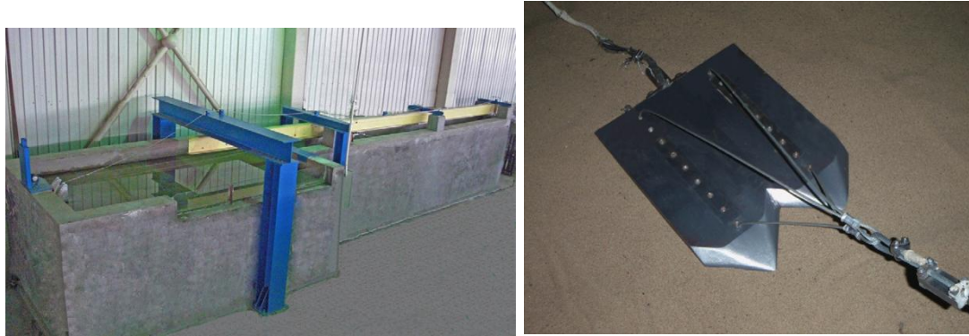
Figure 11. Experimental flume or test tank (left) and the used anchor model (right) (adapted from Liu et al., 2010a)
