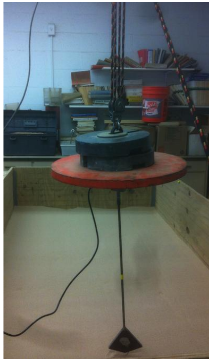
Figure 27. Photograph of the test anchor for the in-plane shear (vertical fluke) test with all weights.
