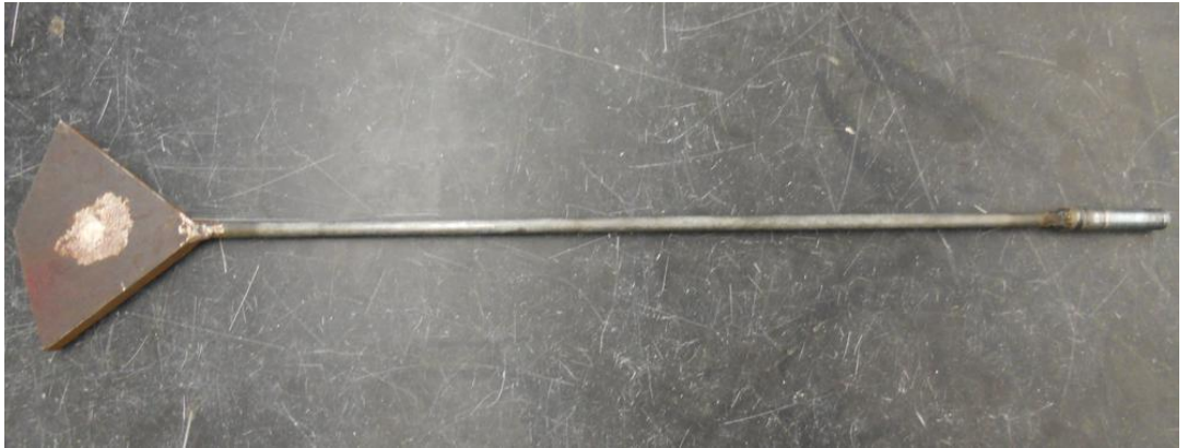
Figure 26. Photograph of the anchor model with attached rod.
