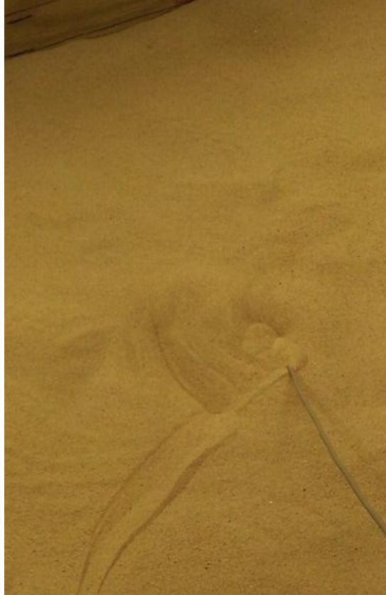
Figure 61. Photograph of the failure surface from the H/B=1 test after rotation.
