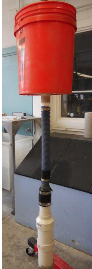
Figure 20. Photograph of the portable pluviator developed by Giampa (2014) and Dietrich (2014) and adapted from Gade et al. (2013).
