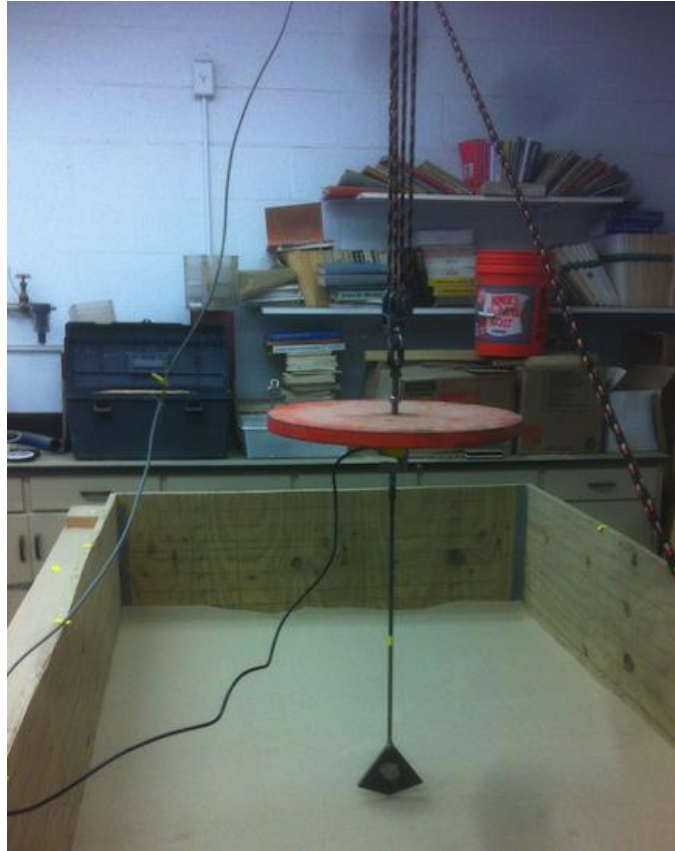
Figure 28. Photograph of the test anchor for the in-plane shear (vertical fluke) with reduce weight.
