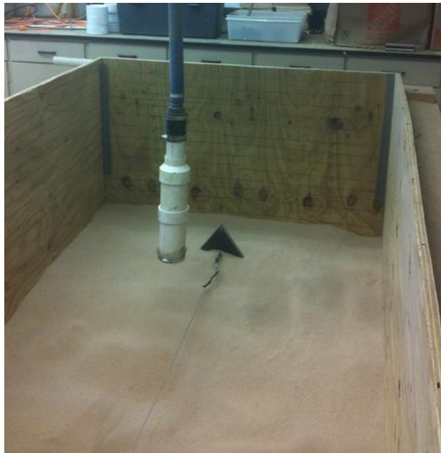
Figure 35. Photograph of the test anchor for the normal (vertical fluke) tests.
