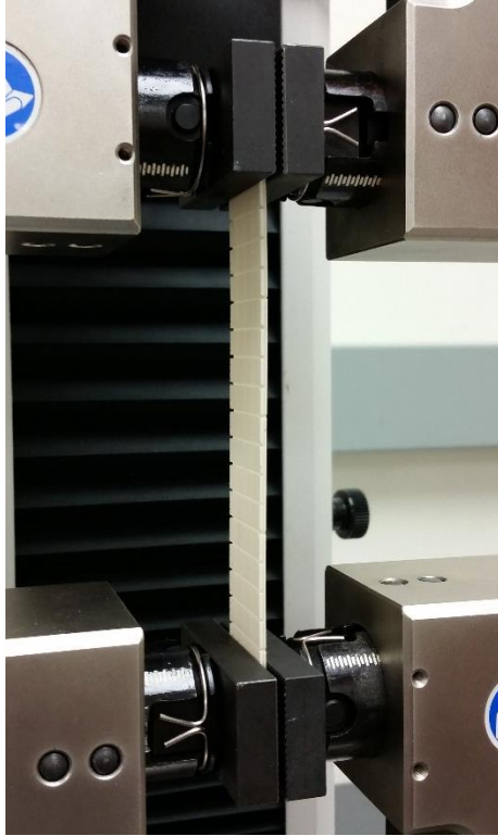
Figure 19: Tensile Experimental Setup for the IC1000 Pad
