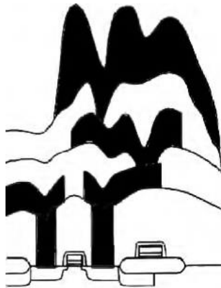
Figure 5: Layer Representation of an IC Fabricated without Planarization (Li 2008, 734)
