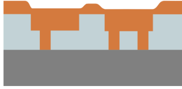
Figure 4: Wafer Cross Section after Metal Deposition
