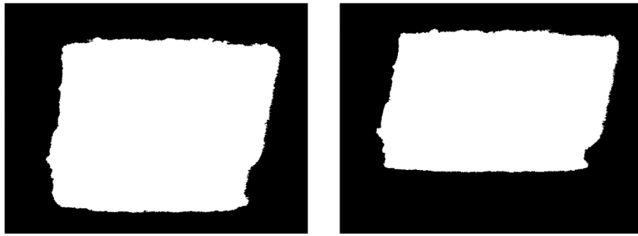
Figure 16: Rotated Binary Images of Pad Sample. Left: Uncompressed. Right: Fully Compressed.
