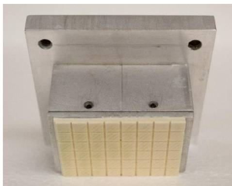
Figure 22: Polishing Pad Tribometer Fixture
