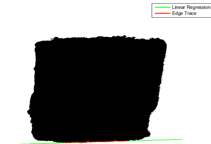
Figure 15: Binary Image of Isolated Pad Sample with Linear Regression for Rotation
