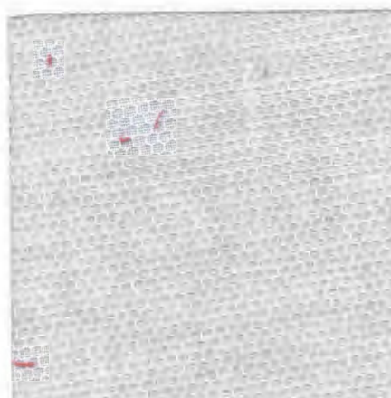
Figure 34. Silk tulle post-abrasion
