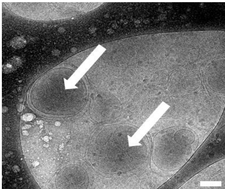
Figure S1 (A) Cryo-TEM image showing effect of addition of 2wt% cyclohexanol to a DEEDMAC vesicle suspension after 24 hrs. Multilamellar vesicles (white arrows). Scale bar = 100nm.
