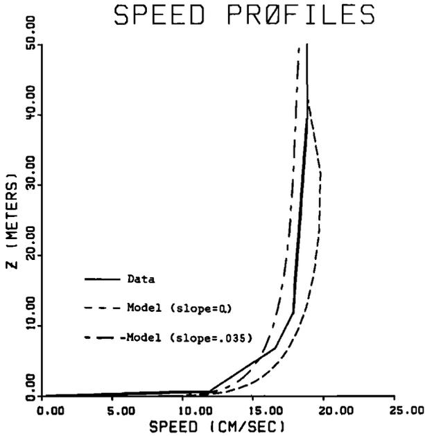
Fig. 10. Observed and model speed profiles. The model profiles were plotted from day 3 of the simulation. The data are average speeds over the 5-day period.
