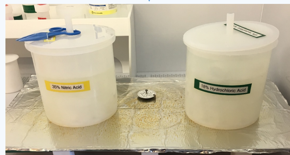
After observing contaminants in our standards, Teflon bottles were cleaned on a 150°C hot plate in 35% nitric acid followed by 18% hydrochloric acid before use
