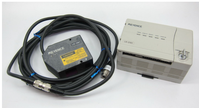
Figure C.5: Keyence LK-081 laser displacement sensor head with laser controller.
