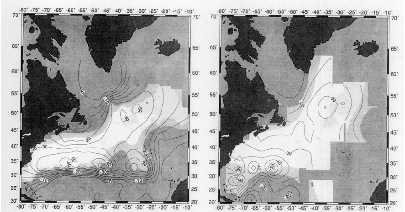
FIG. 6. Contour plot of m_l , 0–3000-db, 5° bins, for (a) CAWO and (b) historic datasets. Contour interval is 5 dyn m s -1 . Corresponding correlations r_m of \Delta D with \tau are shown by shading. Unshaded region has strong correlation ( r_m < -0.9 ). Lighter shaded region has fair correlation ( -0.9 < r_m < -0.8 ). Darker shaded region has poor correlation ( -0.8 < r_m ) or is a region of no data (contours absent).
