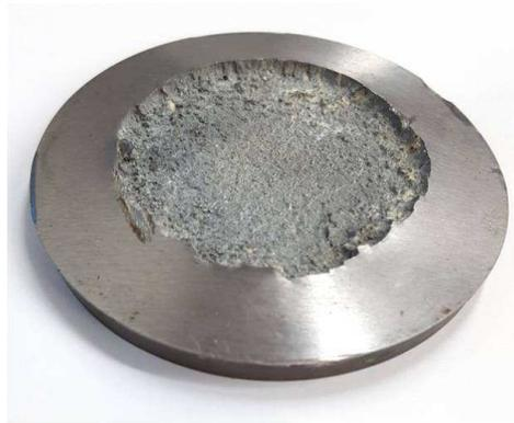
Figure 1-28: Spall fracture in the backing plate from a plate impact test at 12 GPa.
