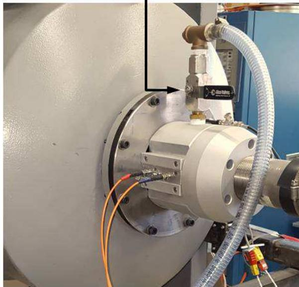
Figure A- 6: Vacuum valve 2 used for evacuating the barrel and target fixture.
