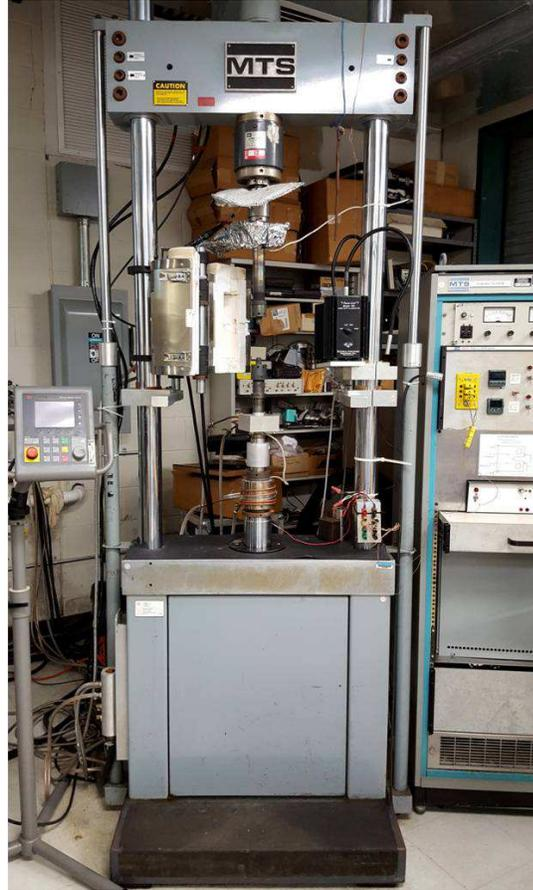
Figure 1-2: MTS machine used for quasi-static tension and compression tests.
