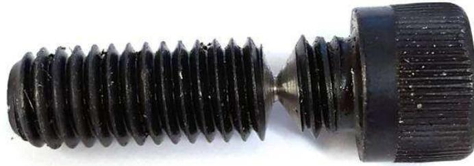
Figure 2-34: 3/8"-16 bolt used for mounting the target to the vacuum chamber. The diameter has been turned down to 1/16in. to reduce the force to break during impact of the specimen.
