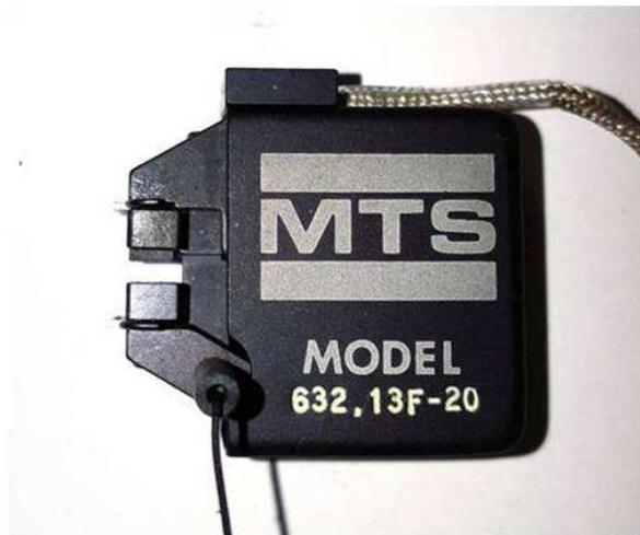
Figure 1-5: MTS model 632-13F-20 knife edge extensometer for quasi-static strain measurements in tension or compression.
