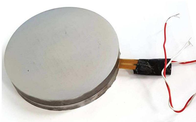
Figure 2-36: Picture of a target specimen ready for testing with the stress gauge bonded and with wire leads soldered to the stress gauge tabs.
