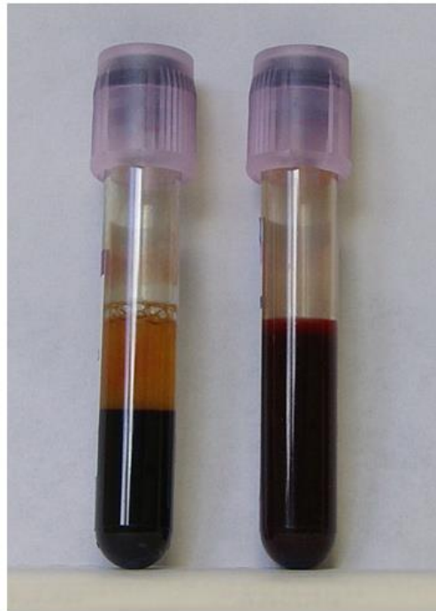
Figure 2-2: Blood separation via centrifugation (left vial) compared to whole blood without separation (right vial)
