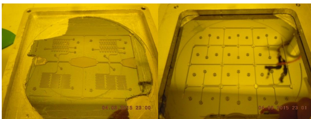
Figure 3-3: Completed silicon wafer molds used for LOC chip production for multi-fluid assays (left) and single fluid assays (right)
