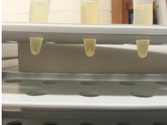
Figure 4-9: Centrifuged serum with ethanol for plasma/serum tests. Note that the middle vial had no ethanol added to it
