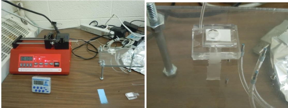
Figure 3-8: Apparatus of syringe pump (left) and PDMS chip (right) used for plasma extraction
