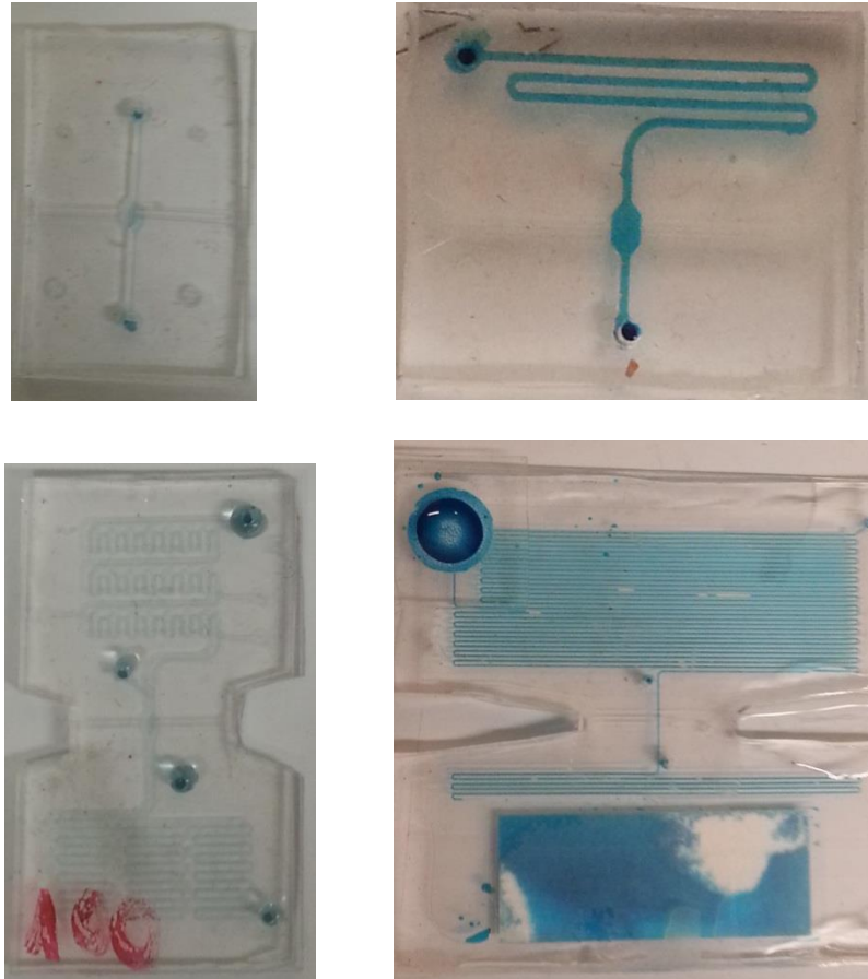
Figure 3-16: Chips used in serum/blood experiments. Clockwise from top left: single-channel detection area, single channel with IgG depletion area, multichannel with IgG and albumin depletion areas, multichannel with multiple IgG depletion areas.
