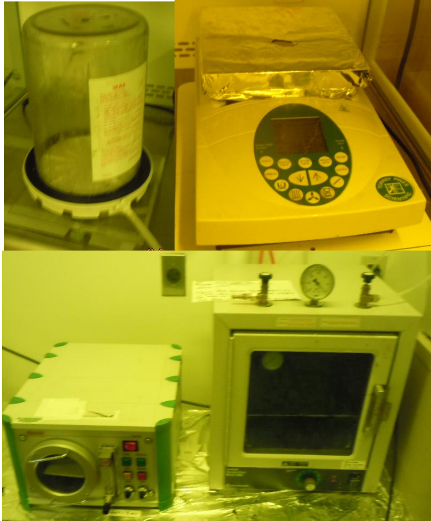
Figure 3-7: Equipment used to create PDMS chips including vacuum chamber (top left), hot plate (top right), plasma asher (bottom left) and vacuum oven (bottom right)
