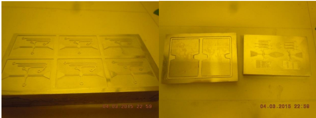
Figure 3-4: Aluminum molds used for LOC chip production for single fluid assays (left) and multi-fluid assays (right)
