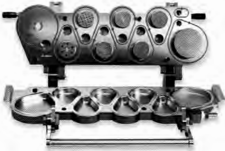
Figure A.6. Next generation impactor (NGI) is a high-performance, precision, particle classifying cascade impactor designed for testing MDIs, DPIs, nebulizers and aerosol and nasal sprays. ( www.mspcorp.com )
