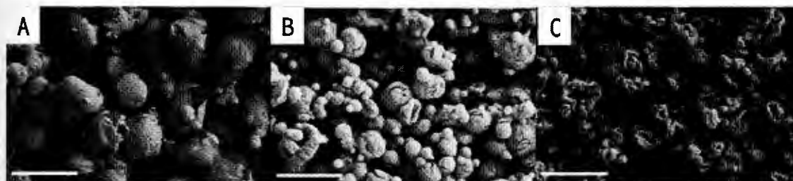
Figure 5.4. Representative SEM micrographs of curcumin-loaded nanocomposite microparticles (CUR nCmP) spray dried with varying conditions such as inlet temperature ( T_{in} ), nanoparticle loading (NP%), and feed concentration (Fc), including: (A) T_{in} = 50\text{ }^{\circ}\text{C} , NP% = 20%, Fc = 1.5%, (B) T_{in} = 90\text{ }^{\circ}\text{C} , NP% = 50%, Fc = 1.5%, and (C) T_{in} = 90\text{ }^{\circ}\text{C} , NP% = 80%, Fc = 0.5%. Scale bar = 5 \mu\text{m} .
