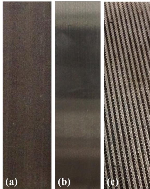
Fig. 1: 1018 mild/low carbon steel specimen with mean roughness index (a) fine [ R_a = 0.8 \mu\text{m} ], (b) grinded [ R_a = 1.4 \mu\text{m} ], and (c) milled [ R_a = 5.0 \mu\text{m} ]
