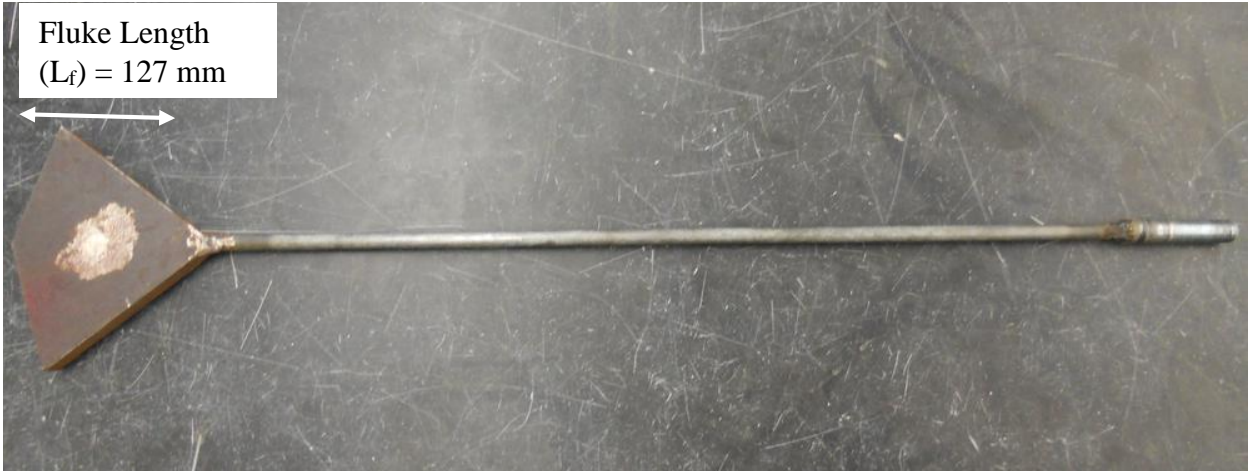
Figure 4.6. Photograph of the anchor model with attached rod used for pure loading of a vertical anchor loaded parallel to the fluke area.
