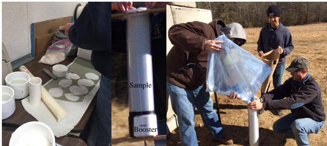
Figure 3.4. Photo Showing Preparation of Booster and Assembled Test Device
