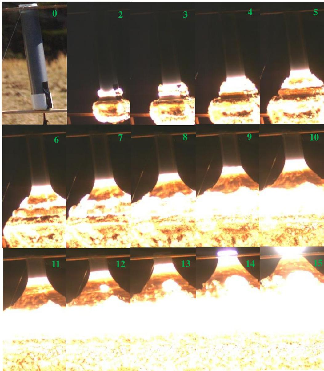
Figure 6.76. High speed camera record from large scale testing with  $\text{NH}_4\text{NO}_3:\text{Al}$  70:30 wt:wt as the sample (20170302 shot 3)
