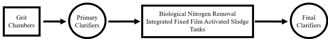
Figure 1. Simplified diagram of treatment train at Field's Point wastewater treatment plant. The figure shows only the components GHGs were measured from in this study.
