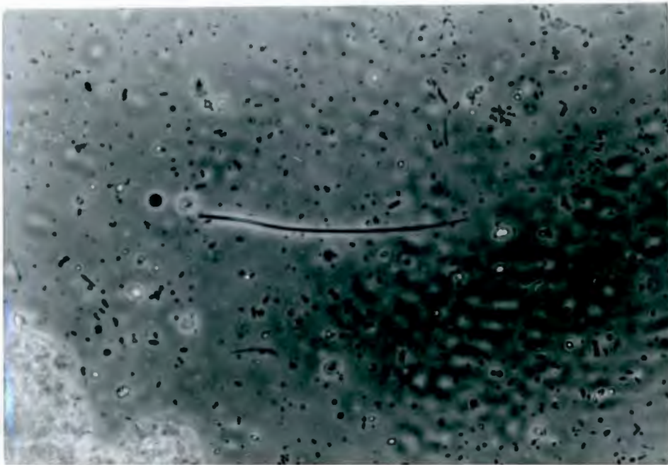
Figure 7.4.1.7 Photomicrograph of dispersed bacteria in the activated sludge (160x)
