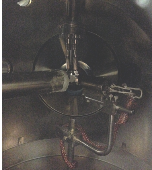
Figure 17. Sample mounted in the chamber using a sample holder, which is made with a tantalum foil folded around tungsten wires.
