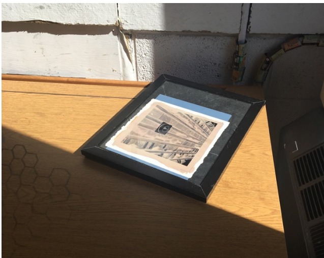
fig. 4 A Vandyke brownprint being exposed to UV light in a contact-printing frame.
