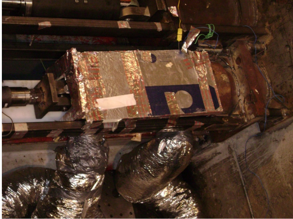
Figure 13 – Size 35 inside the makeshift “oven” during a high temperature functional test. The size 100 can be seen mounted on the large test machine at the top of the photo. Richards, Rick, 2009
