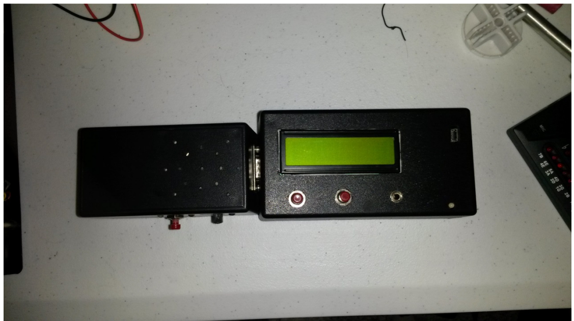
Figure 1. Picture of AAGILE System. Mobile unit is on left. Docking station is on right.
