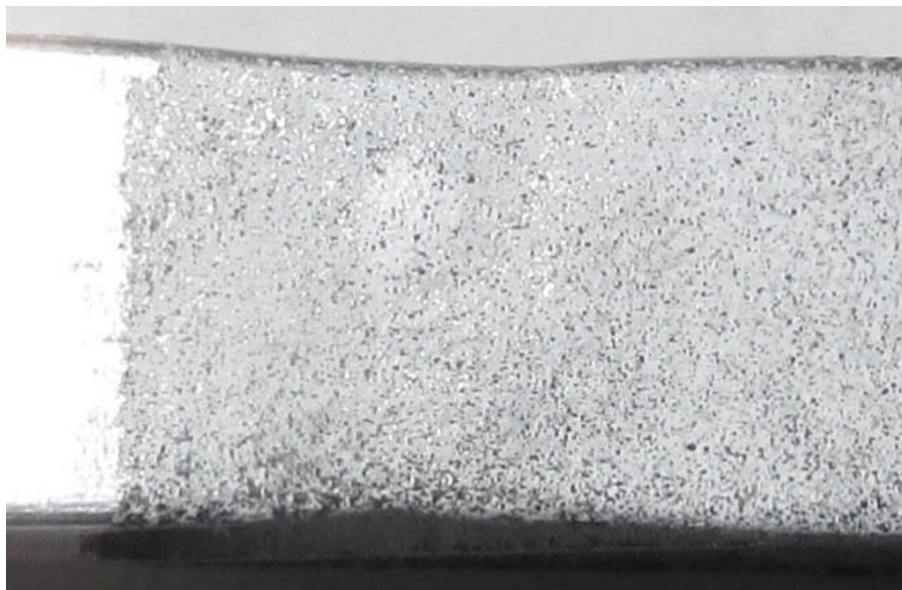
Figure 22 - Sample T2 Member Necking
