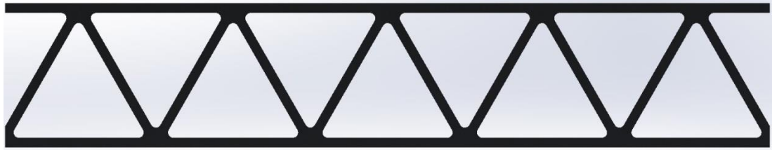
Figure 8- Typical Truss Structure Volume Fraction 0.25
