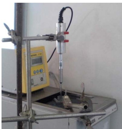
Figure 3.1: Setting probe sonication with probe, cryostat and sample
