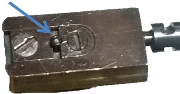
Figure 3.14: cSEM sample holder. Blue arrow points to holder which is used for placing the sample
