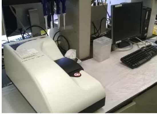
Figure 3.12: Dynamic Light Scattering system and PC- setting
