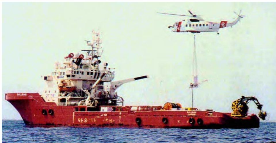
Figure 2.1: A Sikorski 61N helicopter reloading dispersant spray bucket from a support vessel [EMSA, 2009]
