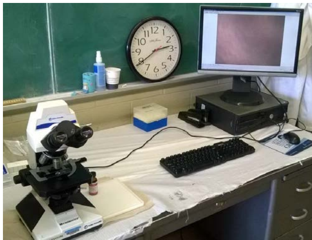
Figure 3.13: Optical microscope with attached PC
