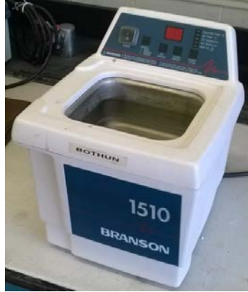
Figure 2.11: Picture of bath sonicator Branson 1510
