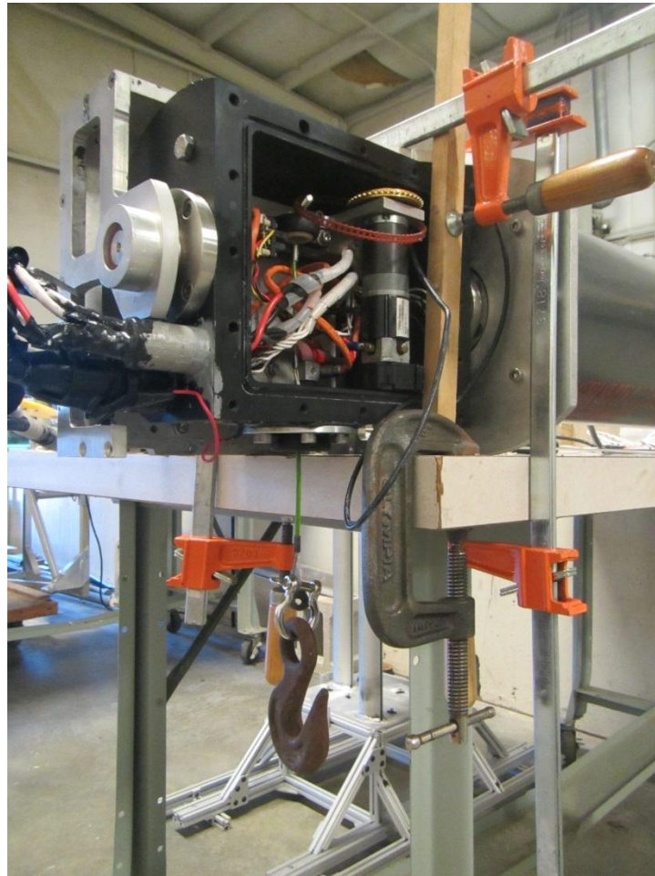
Figure 16. Applying an x-direction force
