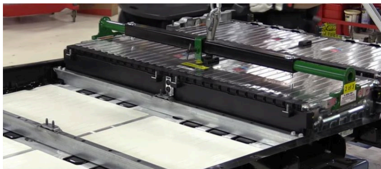
Figure 9: Disassembly step D39, the lifting of four battery modules [12].
