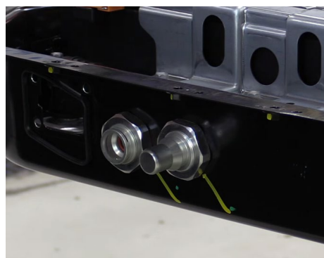
Figure 7: Disassembly step D12, the Big Nuts for Coolant Hoses [12].
