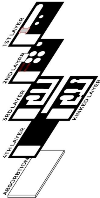
Figure 3-25: Assembly of 3-Fluid Chip (alternate 'Kink' layer is shown also)
