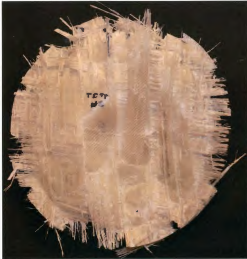
Figure 17: Post-mortem evaluation of Panel B at 0.52 MPa.
