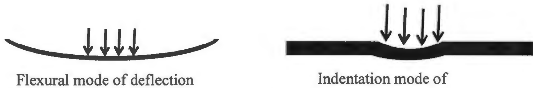
Figure 15: Flexural and Indentation mode of deformation
