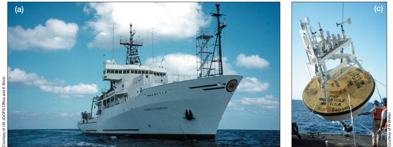
Figure 5. Elements of an interdisciplinary ocean observing system include: (a) commercial and research ship-based surveys and time-series; (b) moorings and coastal and regional cabled networks (eg ORION http://www.orion.org ); and (c) autonomous drifters, floats and gliders, and aircraft and satellite remote sensing (see Figure 4; Doney et al. 2004).
