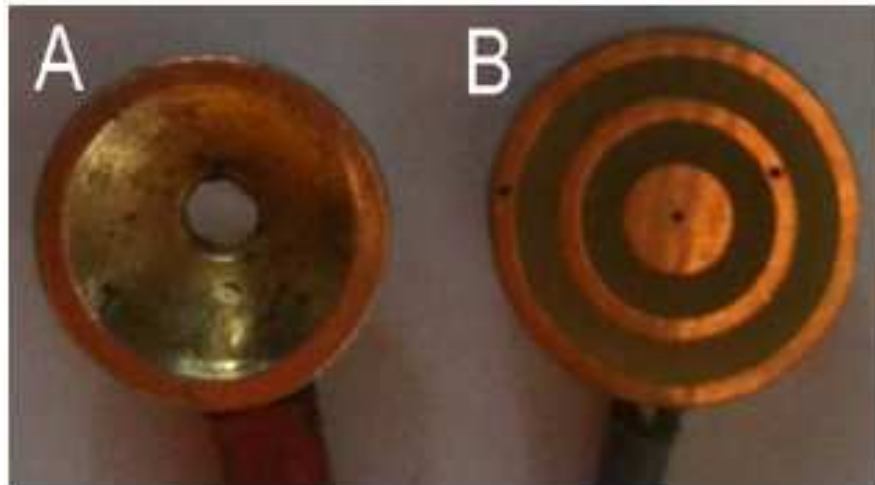
Figure 1.1 Conventional disc electrode (A) and tripolar concentric ring electrode (B)
