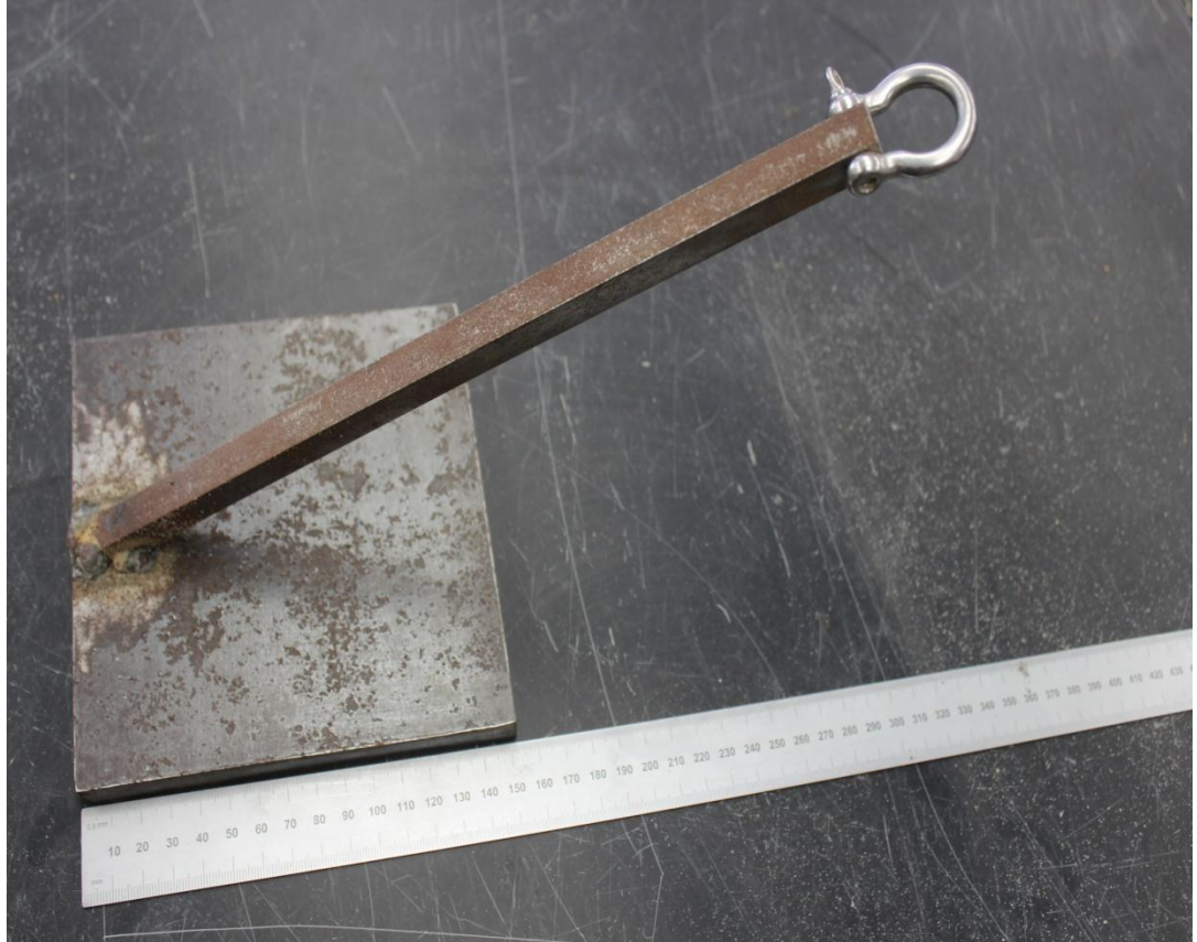
Figure 64- Drag embedment anchor
