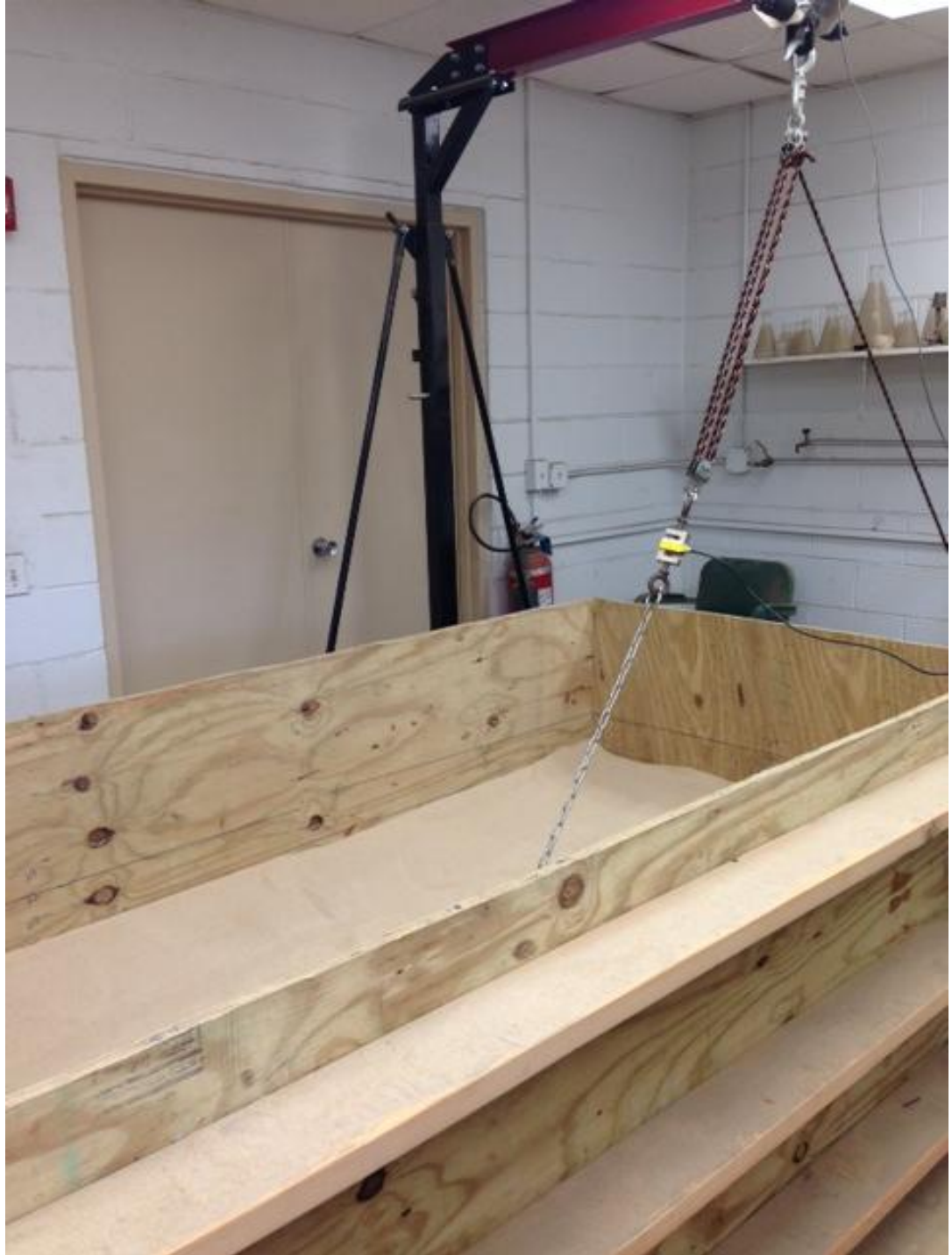
Figure 66- Inclined pullout test setup
