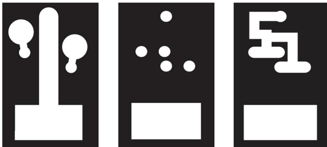
Figure 3-3: Different Layers of the Microfluidic Chip (First Layer, Hydrophobic Layer, Second Layer)
