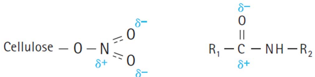
Figure 2-2: Electrostatic binding on nitrocellulose [33]
