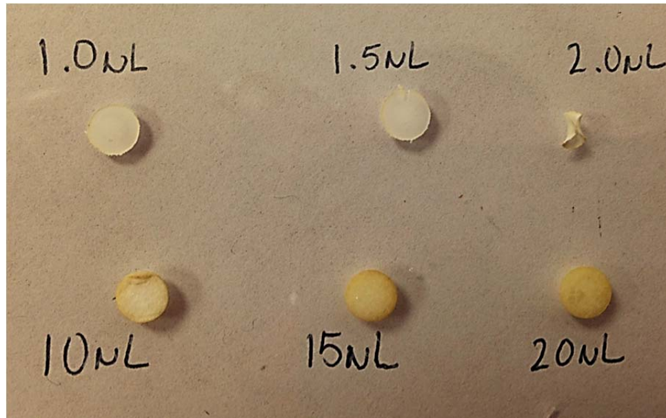
Figure 4-3: Immobilization of Trypsin on Nitrocellulose (Top) and Blotting Paper (bottom)
