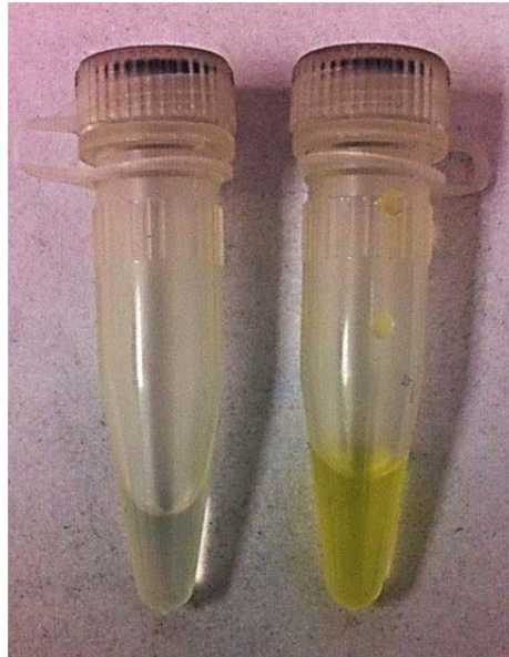
Figure 4-2: Color change in a vial using trypsin and BAPNA
