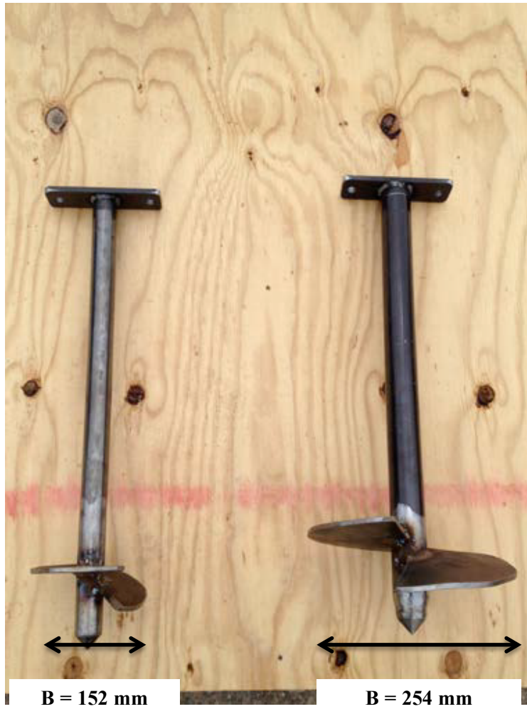
Figure 5: Test anchors ( B = 152 \text{ mm} , Total Length = 597 mm; B = 254 \text{ mm} , Total Length = 616 mm).
