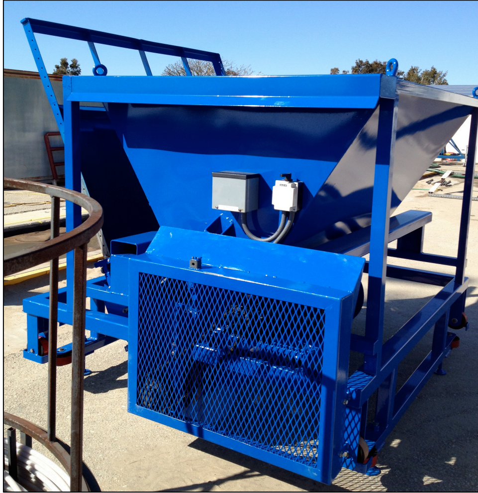
Figure 9: Sand pluviator used for test sample preparation.
