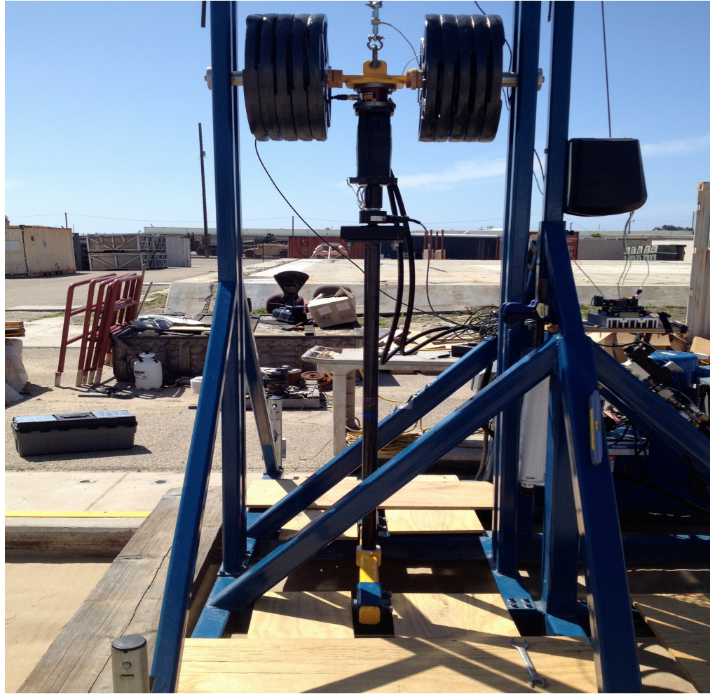
Figure 10: Helical anchor load frame.
