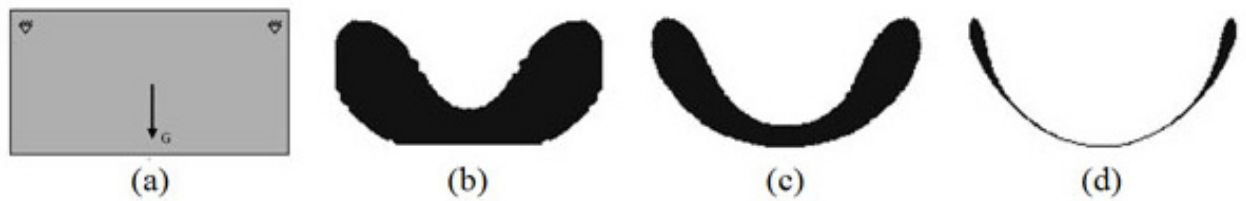
Figure 2.4: A catenary-type structure (a) Initial design (b)-(d) Evolution of optimal shape [17]
