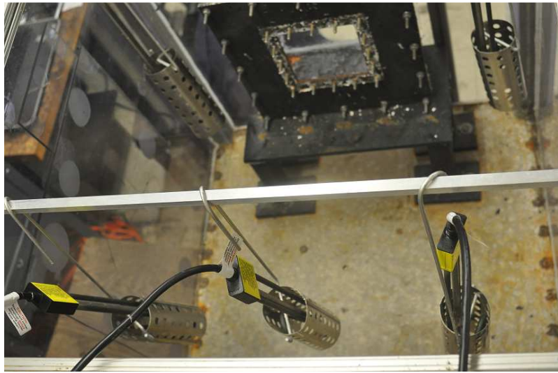
Figure 3.1.6.1-2: Arrangement of the five water heaters
