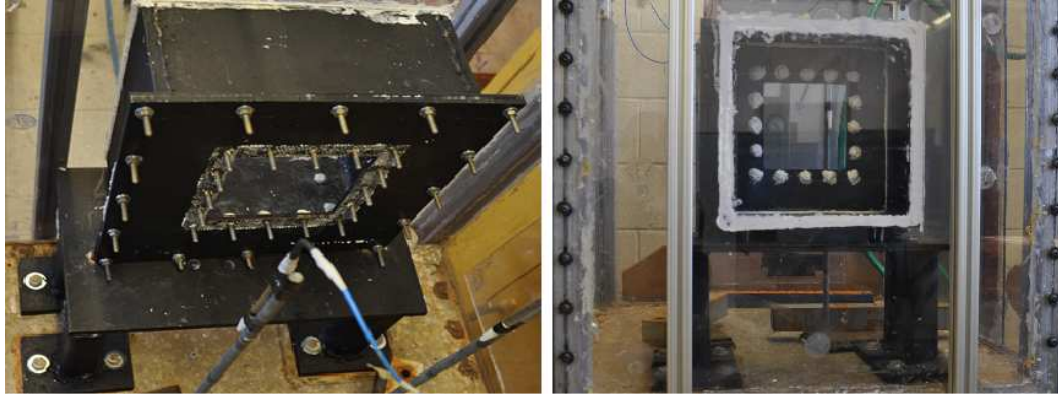
Figure 3.1.2-1: The experimental holding fixture, absent specimen. Left : view from explosive side, showing the mounting screws for the fully-clamped boundary. The white band around the screws is silicone caulking residue, used as a watertight seal between the specimen and the box. Right : view from the DIC side. Notice the thick white bead of silicone between the box and the window, sealing the edges.
