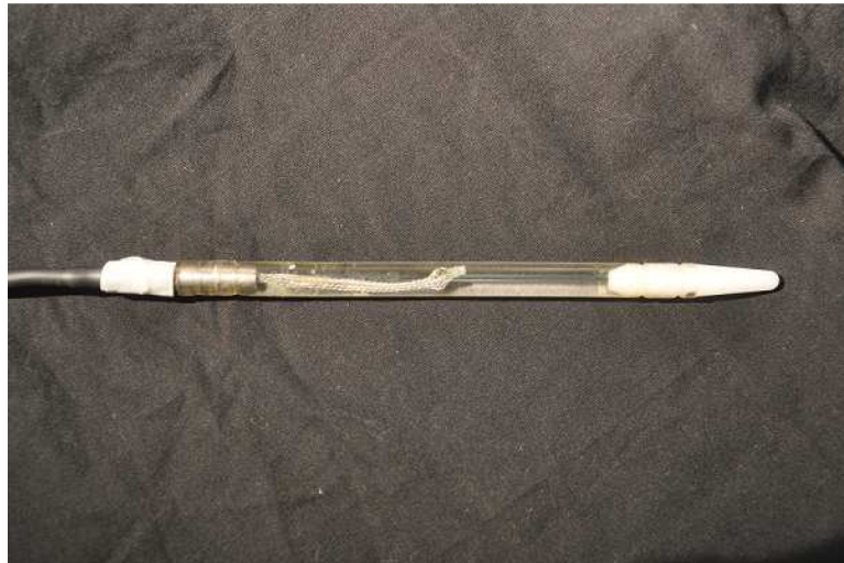
Figure 3.1.3.1-1: Series W138A05 underwater blast probe. The tourmaline sensing element is the spherical shape at the center of the unit. The distance from this element to the end of the conical tip, at right, varied between the sensors.
