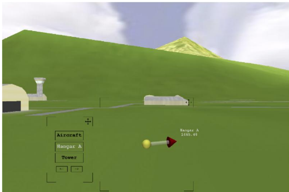
Figure 12: The 3D arrow navigation aid used to point toward targets or places of interest [6].
