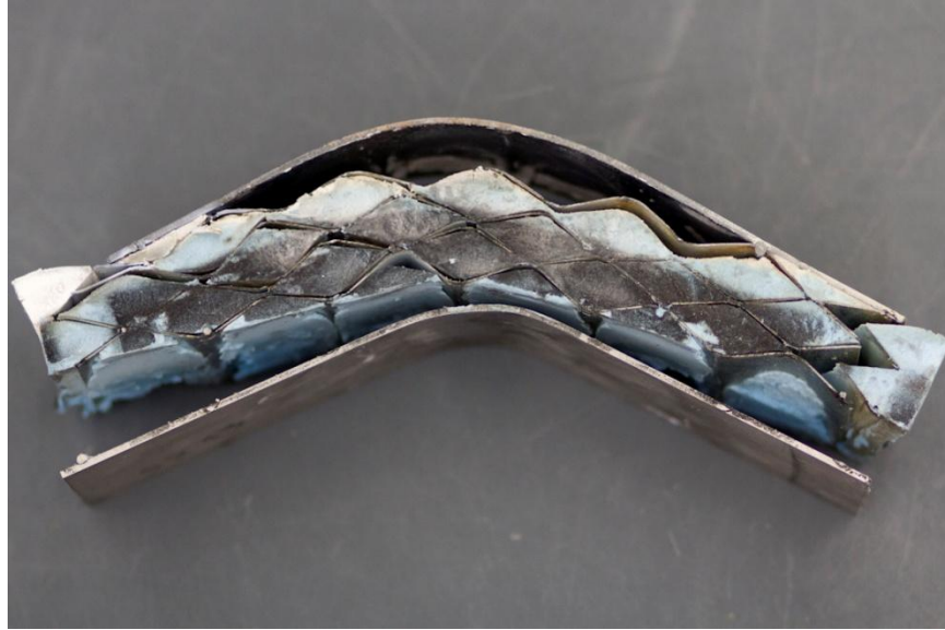
Figure 27- Post-mortem image of 500°C specimen
