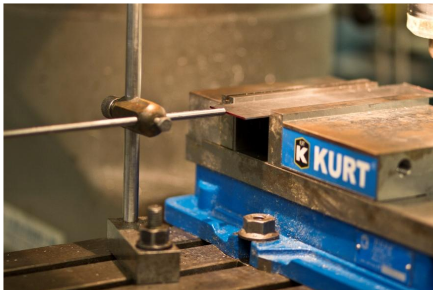
Figure 11. - Image of mill stop positioned at the center of the face sheet
