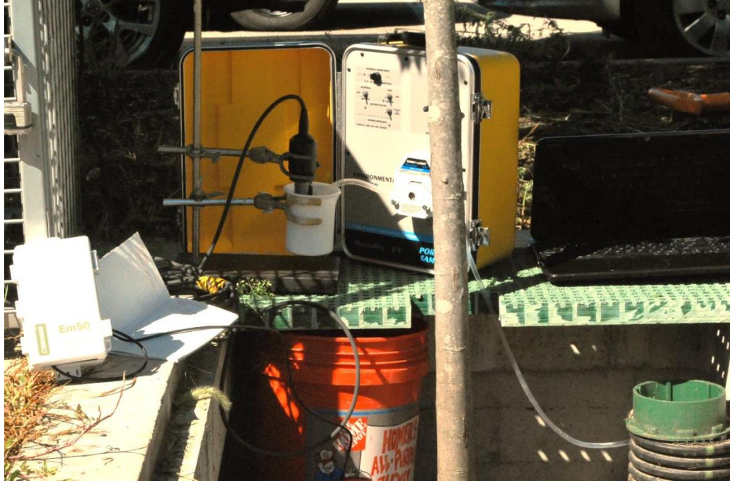
Figure S4.2. Sampling set up during the field tracer experiment. Effluent was pumped up to the surface using the Masterflex Environmental Sampler into a Teflon beaker. The YSI Professional Plus logger was set up to log specific conductivity at five minute intervals. At 15 minute intervals bacteria samples were taken from the effluent.
