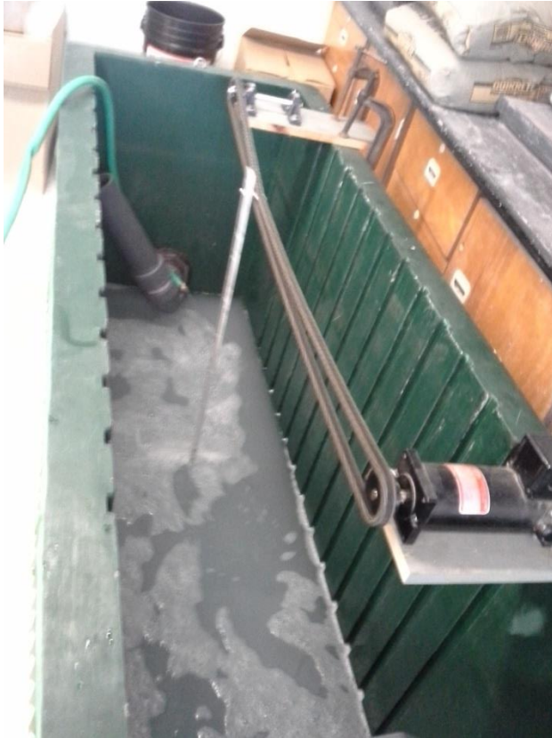
Figure S4.1. Mixing tank used to amend the red cedar wood chips with TPA. The chain has a paddle attached that ensured proper mixing of the solution and the wood chips during the amendment period that lasted 9 days.
