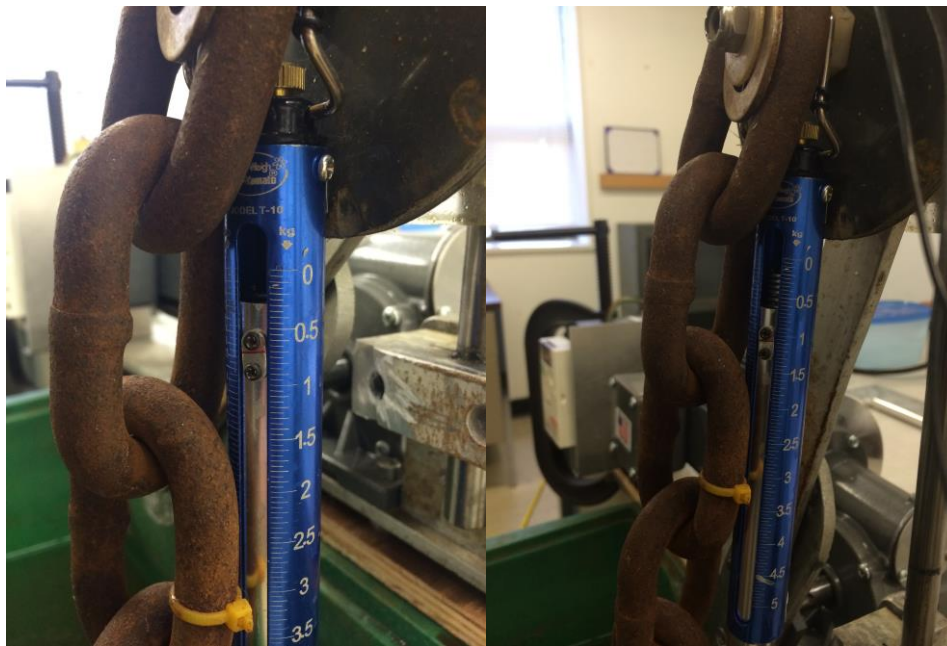
Figure 4.12: Determining tension within chain. Right: up stroke, Left: down stroke.
