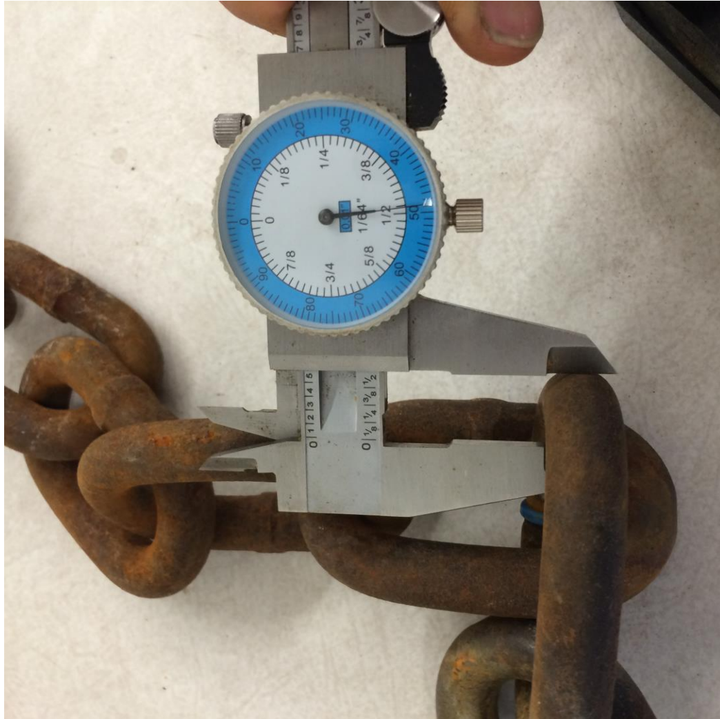
Figure 4.3: Measuring chain wearing surface with calipers
