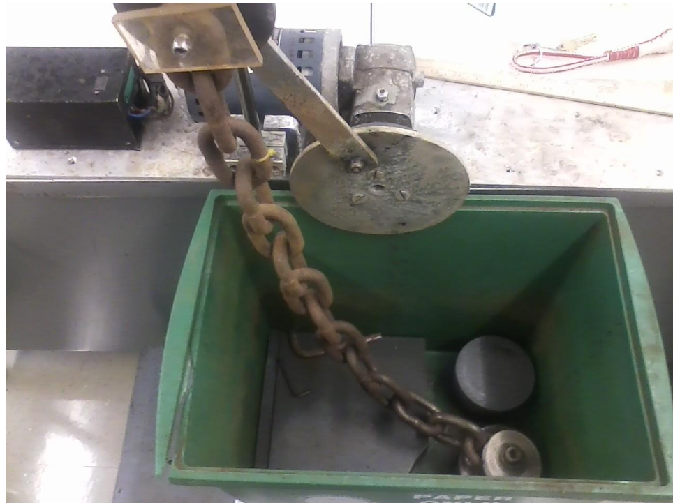
Figure 3.2: First experiment, chain attached to motor via slide apparatus.
