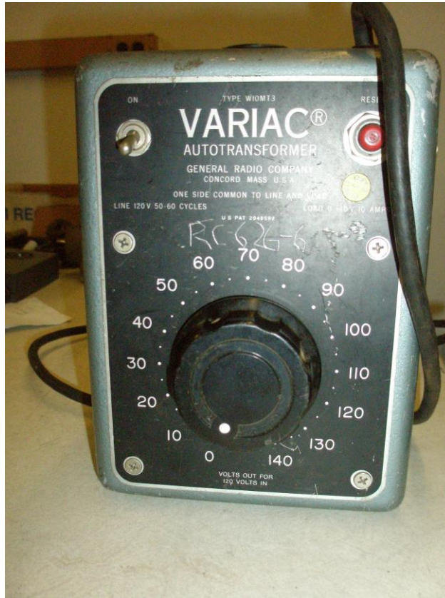
Figure 3.1: Variac used to slow speed of motor in the first experiment.
