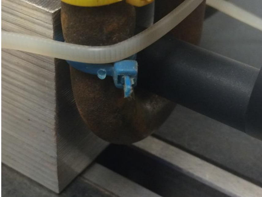
Figure 4.8b: Roughness measurement (Note: orientation of yellow and blue zip ties consistent through each experiment to ensure correct wear surface is measured)
