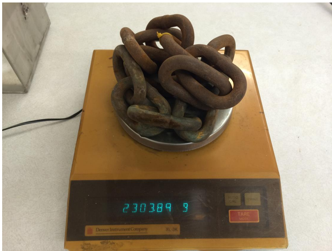
Figure 4.6: Scale used to measure mass of chain.
