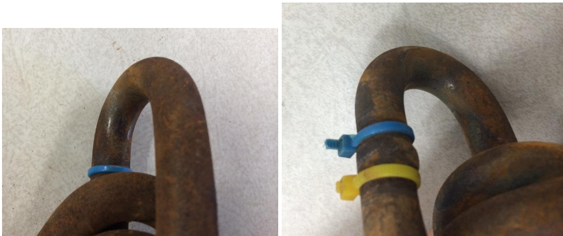
Figure 4.8c: Wear Surfaces. (left) surface at end of second round, (right) surface at end of fourth round.
