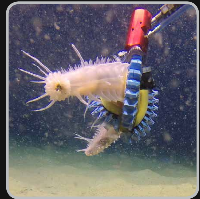
Figure 1. A soft robotic hand is used to collect a holothurian from the seafloor at ~1,800 m in Arguello Canyon, California. The specimen was gently released, with no observed damage to the animal. Photo credit: B. Phillips
