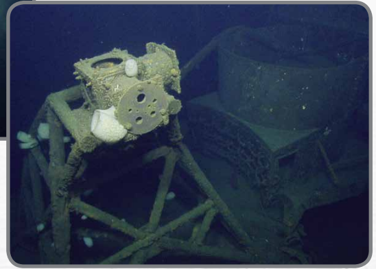
Figure 4. A peak overpressure gauge tower used to mount test instruments at Bikini remains in place at the bow of Independence .
