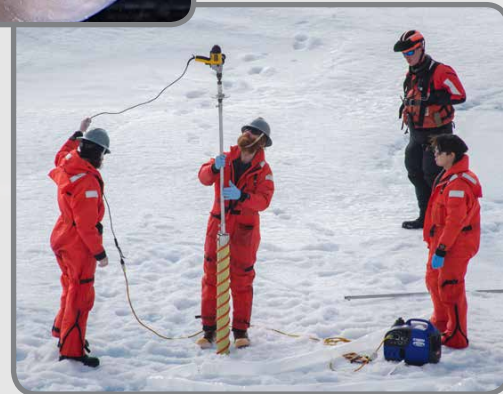
(right) Eric Collins handles the corer with Kyle Dilliaine and Brian Ulaski. The collected ice cores can be seen in the plastic tubing at the bottom of the frame. Photo credit: Caitlin Bailey, GFOE
