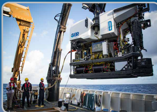
Okeanos Explorer crew deploys NOAA's remotely operated vehicle Deep Discoverer .
