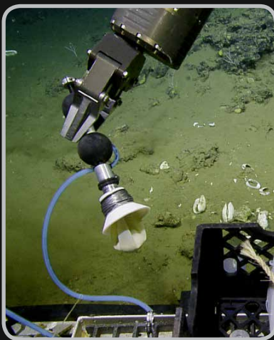
Figure 2. A “jamming” gripper is readied to collect a clam shell on Kimki Ridge at a depth of ~1,200 m.
