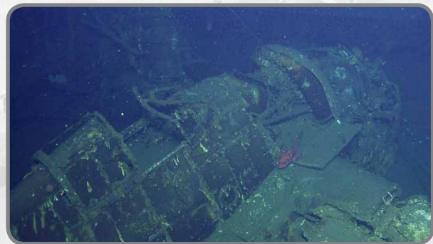
Figure 5. The forward elevator contains a damaged F6F-5N Hellcat fighter placed aboard the ship for Operation Crossroads testing.
