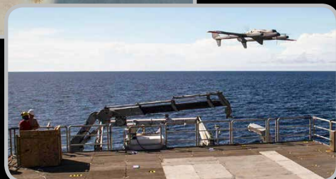
(top) Joe McDaniel integrates scientific instruments into the UAVs. The data collected will provide information about processes affecting air-sea exchange. (bottom) UAVs carrying scientific instruments took off from a ship ( Falkor ) for the first time, without the help of any catapult or launching system. It was also the first time the HQ-60B model completed a science mission. Photo credit: SOI/Monika Naranjo Gonazles
