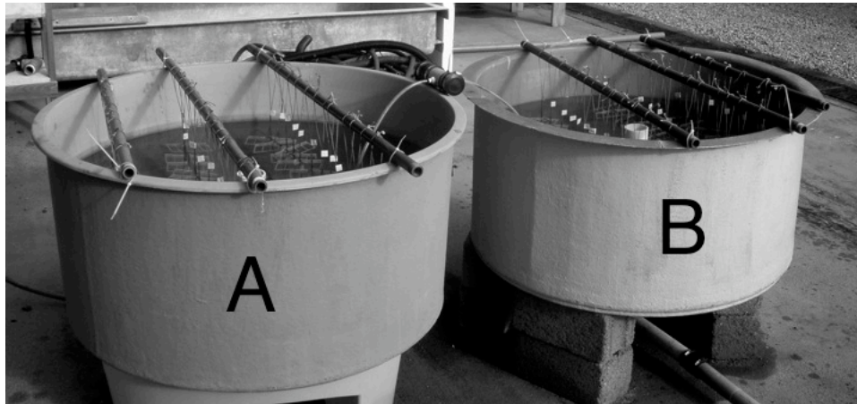
Figure 1. Both summer and winter experiments were set-up with (A) control surfaces and (B) treated surfaces in two separate tanks. Water from Narragansett Bay entered the tanks via the shared pipe located between the tanks. Surfaces were suspended vertically in slide holders hanging by strings in the tanks.
