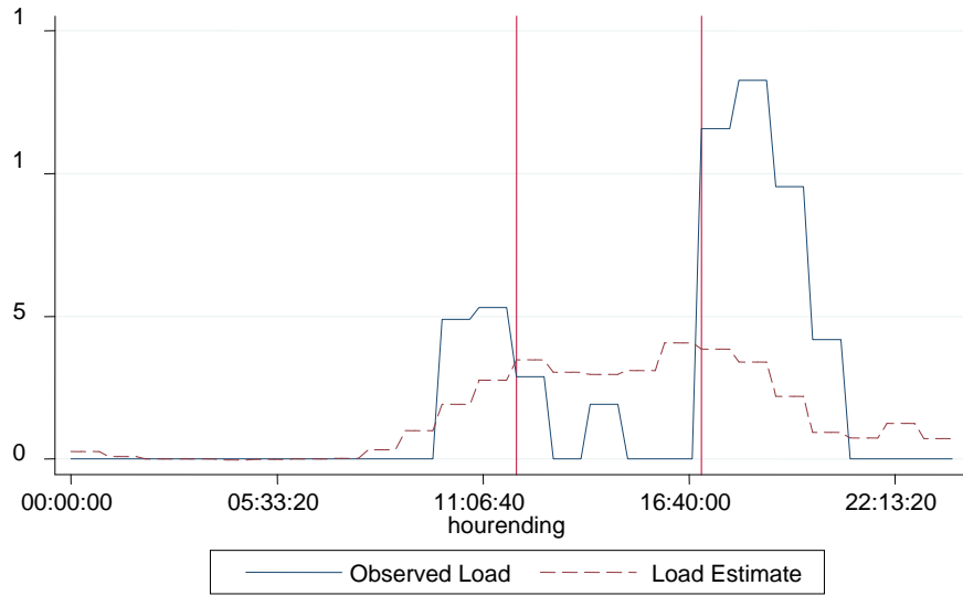
Figure A4-1: Curtailment Day Observed Load vs. Estimated Load
