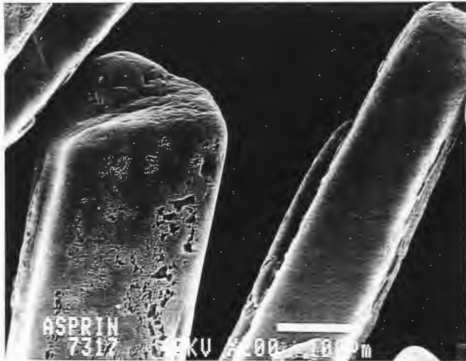
FIGURE 7 : Scanning electron micrographs ( magnified 200 and 3000 times ) of aspirin microencapsules
