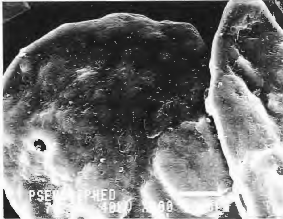
FIGURE 9 : Scanning electron micrographs of pseudoephedrine hydrochloride ( magnified 200 and 3000 times ) microencapsules
