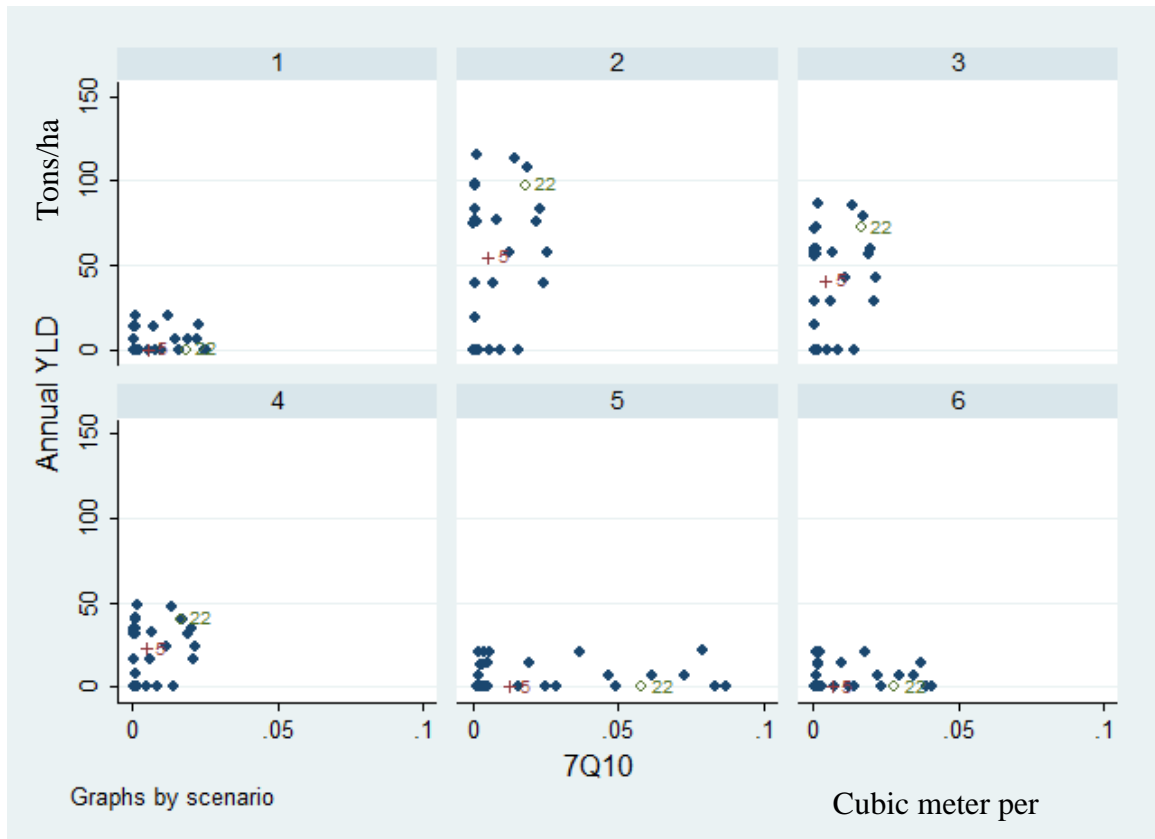
Figure 2. Tradeoff between Crop Yield (vertical axis, annual yield of crop, unit Tons/ha) and Environment Flow (horizontal axis, 7Q10, unit Cubic meter per second) in Different Scenarios; Scenario 1 to 6 represents: Baseline, Conventional Agriculture, BMP Agriculture, Bio fuel, Suburban Medium Density and Suburban Medium Low Density respectively.
