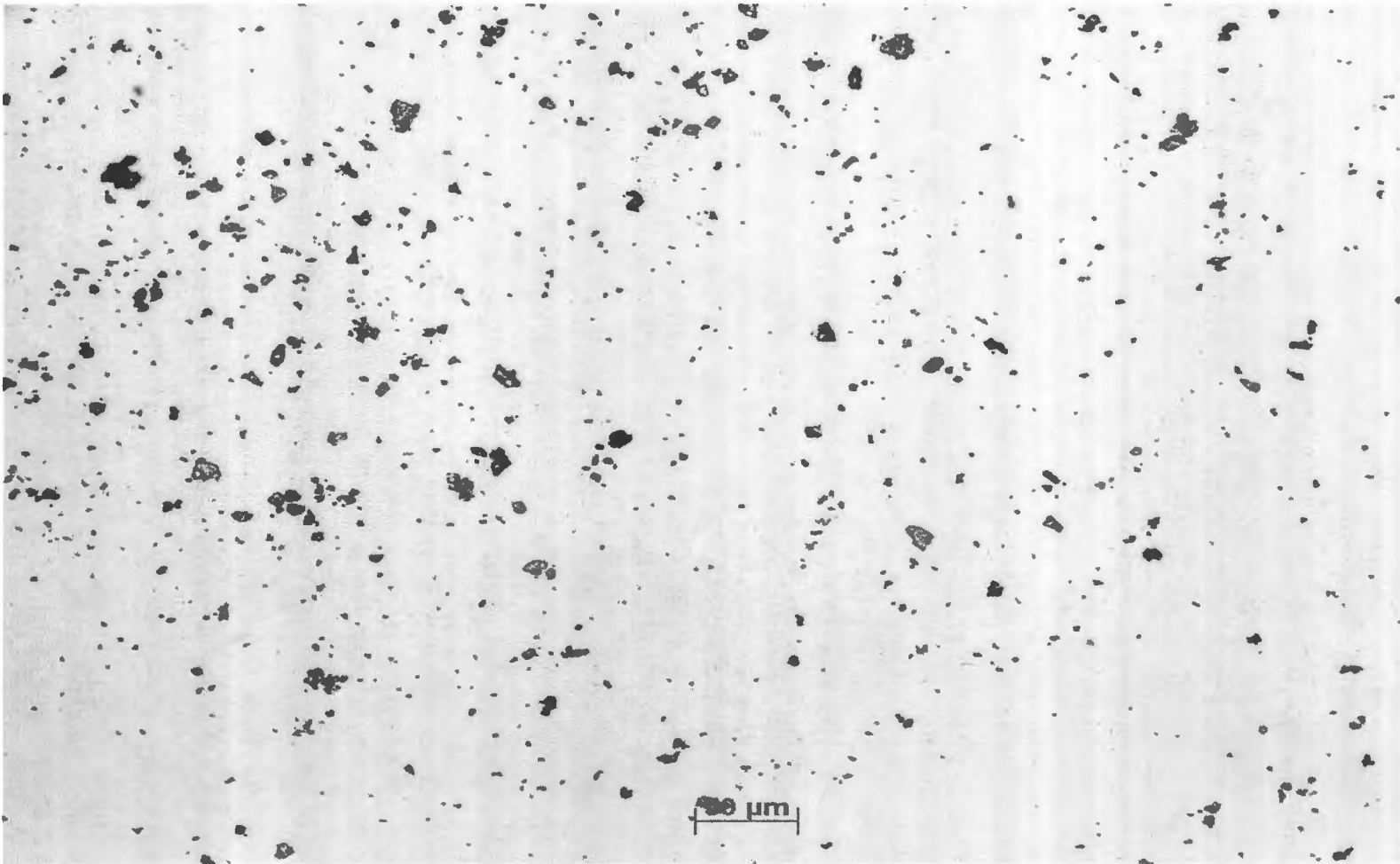
Figure 23: Optical microscopic image of treated cefuroxime axetil showing loss of needle shaped crystals
