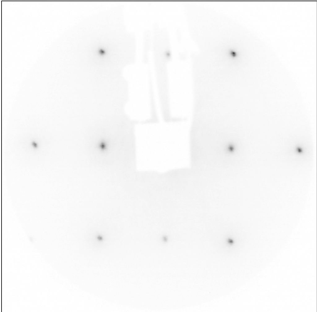
Figure 1-2: LEED pattern observed for Ni(110) after 1 min. of sputtering by 500 eV \text{Ar}^+ at p=2 \times 10^{-7} Torr. The sample temperature was held at \sim 170 K throughout.
