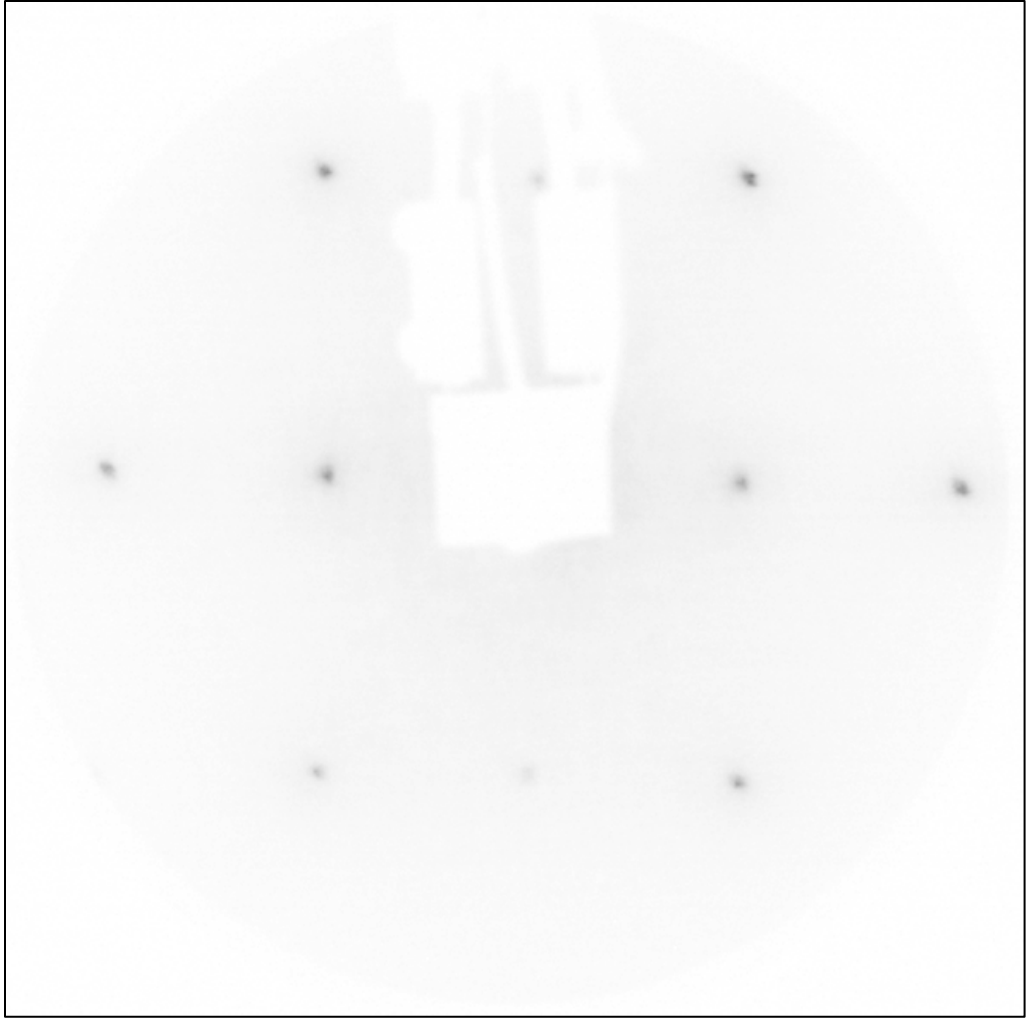
Figure 1-5: LEED pattern observed for Ni(110) after 9 min. of sputtering by 500 eV \text{Ar}^+ at p=2 \times 10^{-7} Torr. The sample temperature was held at \sim 170 K throughout.
