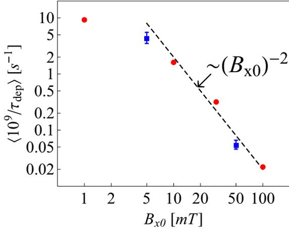
FIG. 1. Comparison of spin flip loss rate calculated in Ref. [21] for the Los Alamos UCN $\tau$  trap [20] using a 1D field model (blue squares) with the present 3D calculation for the smooth field given in Eq. (5) of [20] (red circles). In the range  $B_{x0} \gtrsim 5$  mT the data are represented reasonably well by the power law  $\langle 1/\tau_{\text{dep}} \rangle \sim B_{x0}^{-2}$ , as shown by the dashed line.
