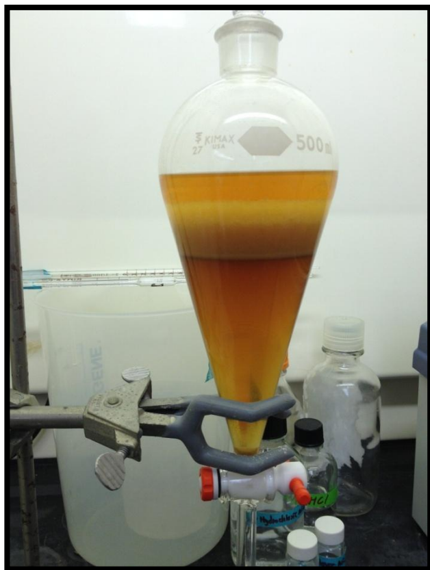
Figure 3. Water saturated n-butanol and soy molasses mixture (1:1, v/v). The three subfractions from top to bottom are butanol phase, interphase and water phase.
